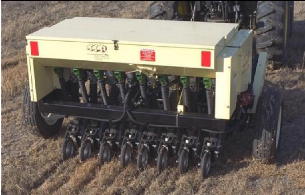
**Figure 22.** A Truax FLEXII no-till rangeland drill. There are eight drill rows on this planter, but they range from 6-22 rows depending on the unit purchased. This drill was used for the CSU revegetation plots at DEN.
