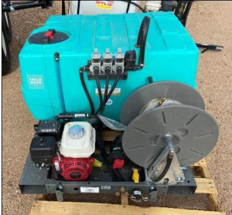
**Figure 15.** This spray unit can be positioned in the bed of the DEN trucks. It can be equipped with a boom sprayer and is currently set up for hand-gun applications with a 100-gallon tank.
