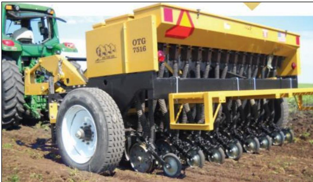
**Figure 23.** Truax OTG rangeland drill is another option for DEN to utilize for in-house seeding work. The number of drill rows range from 8-22.
