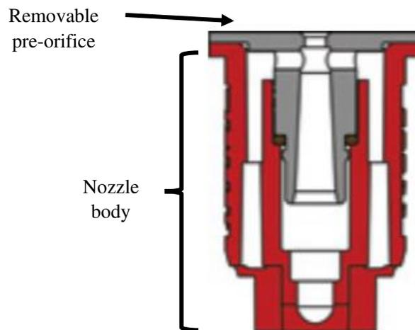
**Figure E3.** TeeJet XR 11003 nozzle body. The grey colored part of the nozzle is the pre-orifice that can be pulled out of the nozzle body. To clean the nozzle, use a soft brush to clean the tip of the nozzle body and pre-orifice.
