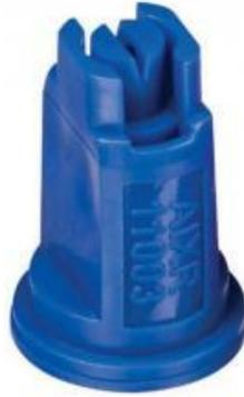
**Figure E1.** TeeJet AIXR 11003 air induction, flat fan nozzle (110 is the wide flat spray angle; 03 represents 0.3 gallons delivered per minute). This spray nozzle is recommended for DEN to use on their 3-point hitch sprayer.
