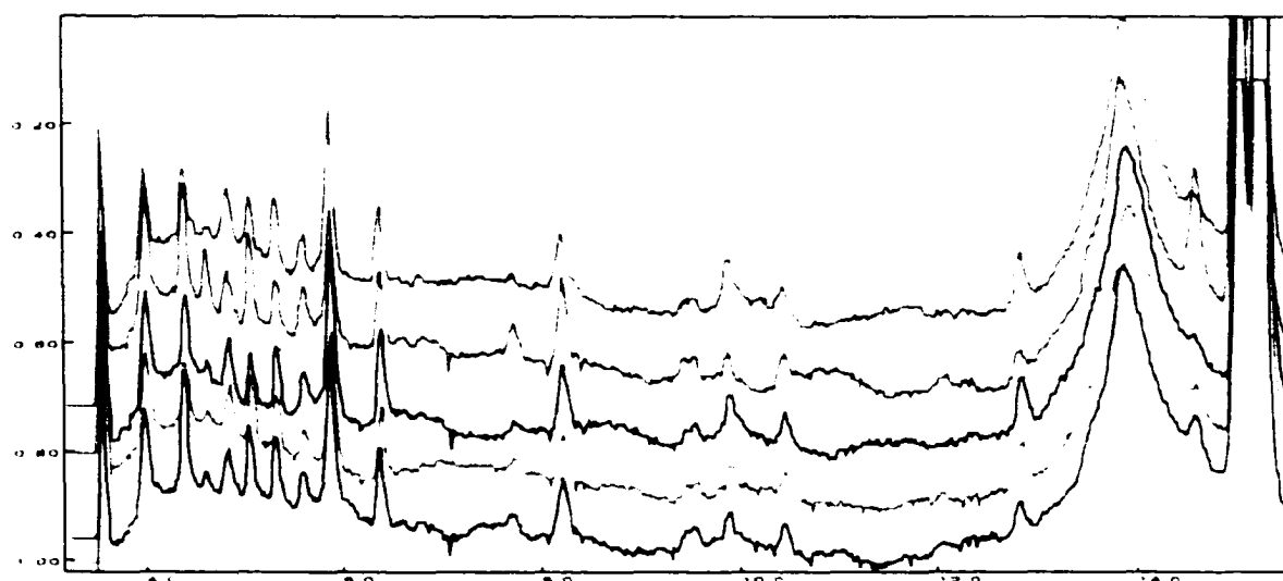
Figure V-3 Chromatogram of PTH-amino acid separation by HPLC in a N-terminal sequencer. This represents the combined chromatogram of five separate cycles of PTH-amino acid separation. Cycles are numbered from the bottom (cycle 1) to the top (cycle 5). By comparing previous and current chromatograms, peak that differs significantly from a previous trace represents a corresponding amino acid residue.
