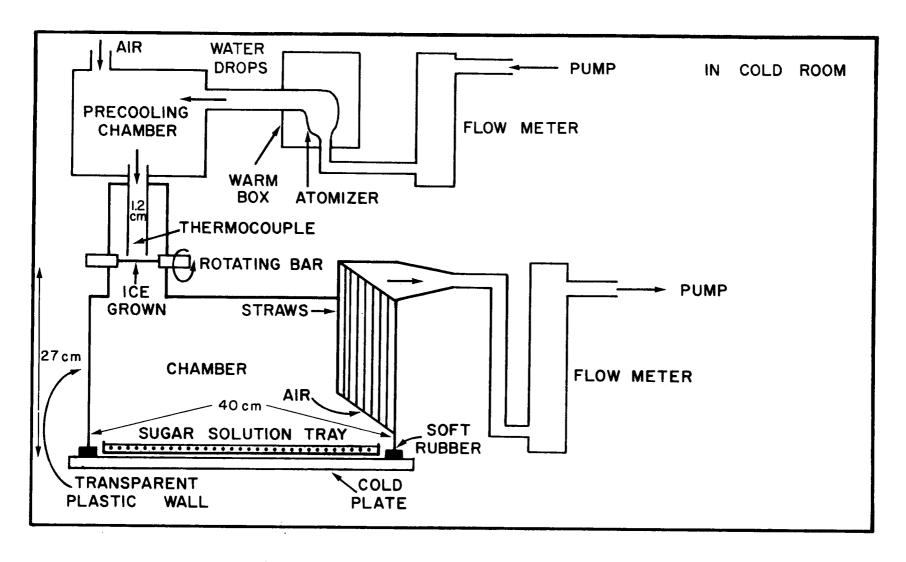
Figure 2-1. Schematic diagram of experimental system.
