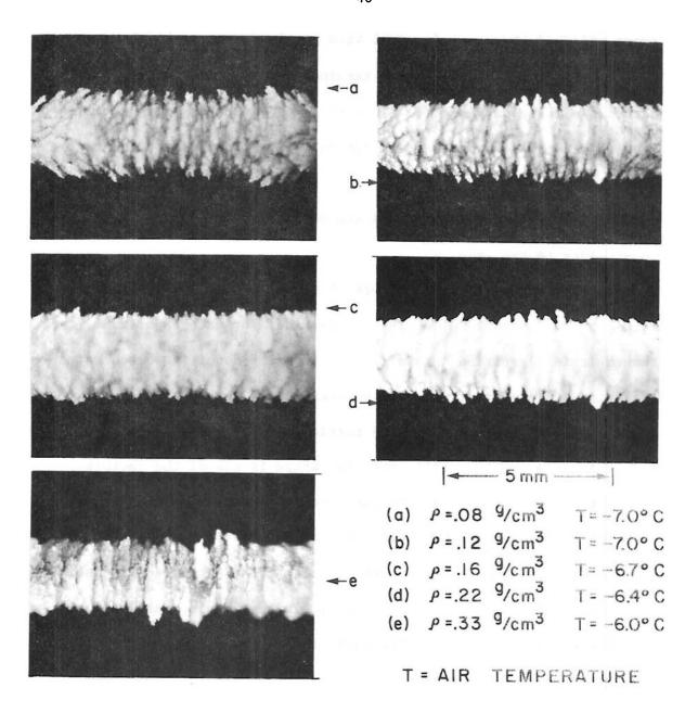
Figure 3-3. Photographs of ice cylinders grown on a rotating bar.
