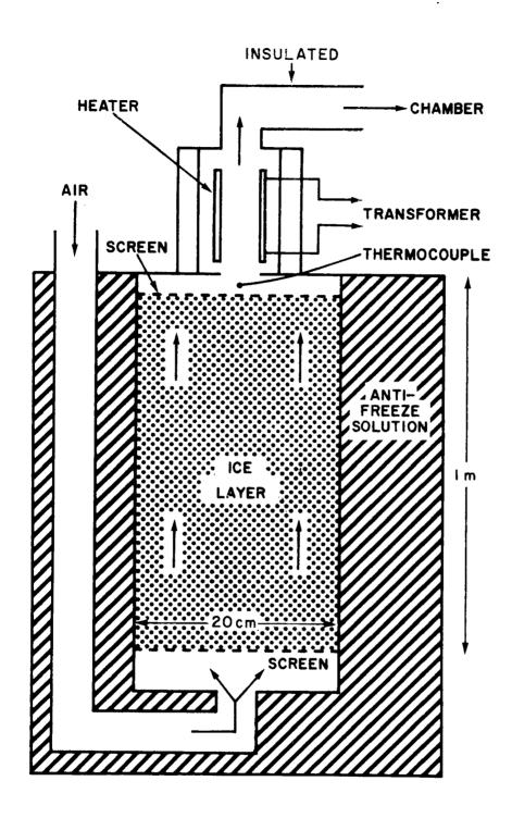
Figure 3-1. Schematic diagram of ice layer used for obtaining a desirable subsaturated air.
