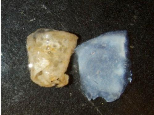
**Figure E1:** DBM-reinforced gels. DBM in the gel at left has denatured due to curing under an uncontrolled temperature profile. At right, a gel cured at 45°C for 12 hours.
