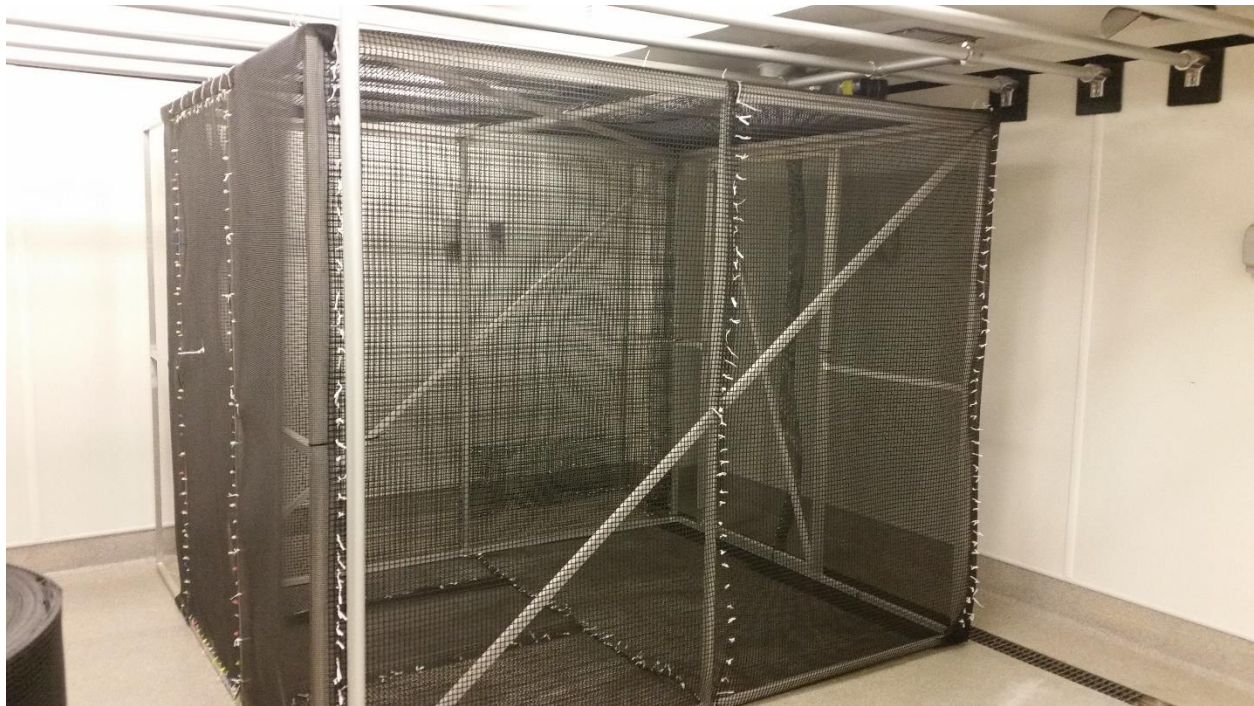
Figure 3.1. Free-flight enclosure constructed for timecourse experiment, measuring 10'x10'x7' to allow for bats to move freely about and forage for fruit. The purpose of building this enclosure was to further optimize husbandry conditions and ensure that any background pathology or stress-induced pathology experienced due to housing or transfer from the colony was minimized during the timecourse experiment.
