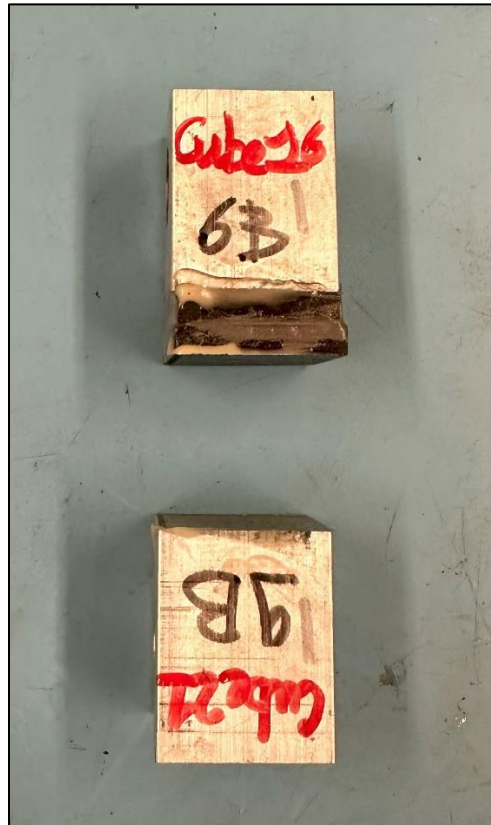
Figure 60. Failed pristine flatwise tension coupon.
