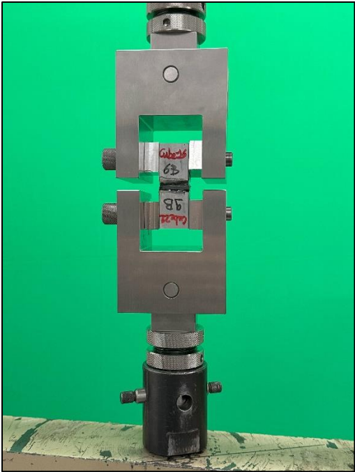
Figure 59. Pristine flatwise tension coupon in the test machine.
