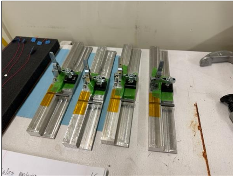
Figure 41. Flatwise tension coupon bond fixture.
