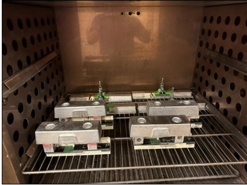
Figure 42. Coupons placed in the oven for the accelerated cure.
