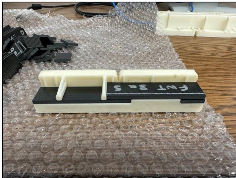
Figure 40. Single lap shear adherends fit into bond fixture.
