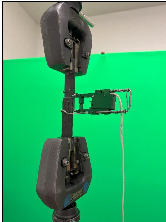
Figure 52. Coupon 1 loaded in the test machine.
