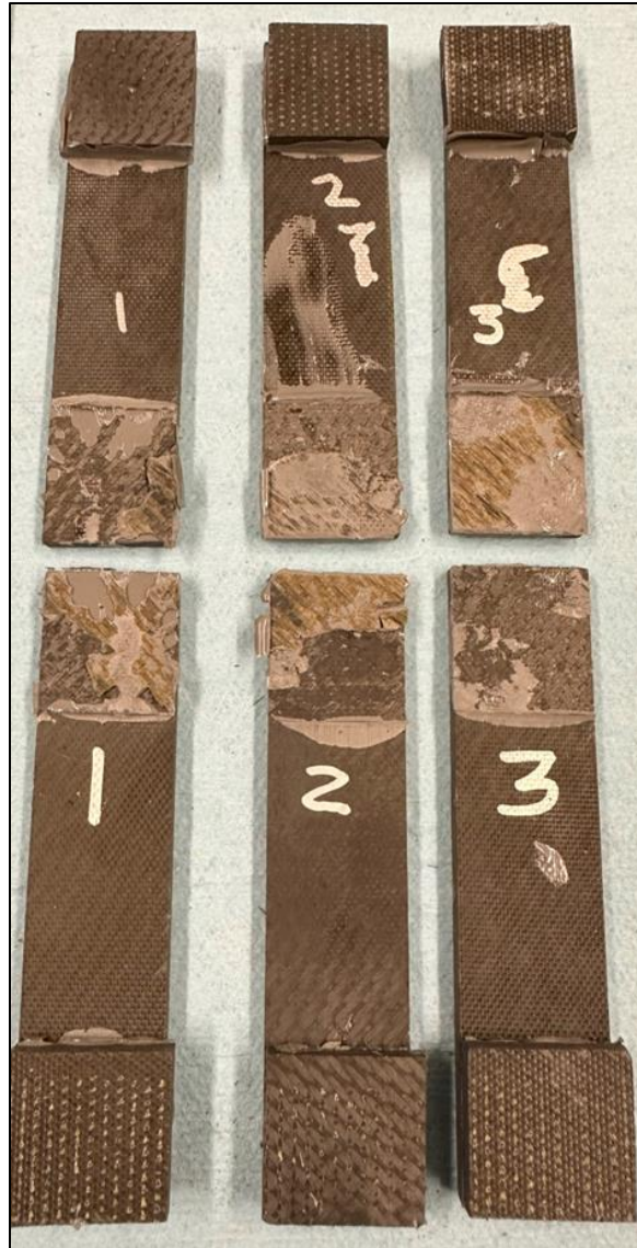
Figure 53. Failed pristine coupon adherends.
