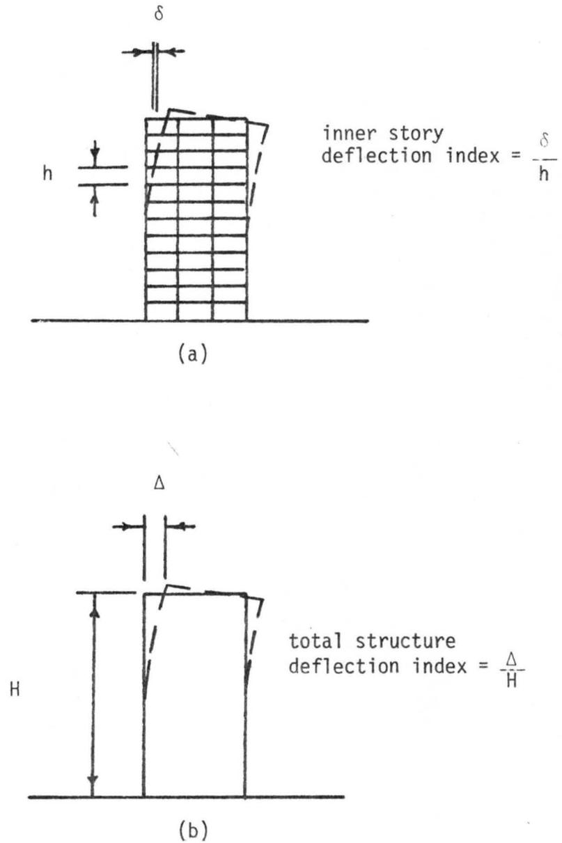
Figure 2.4 Inner story deflection index (a) and total structure deflection index (b).
