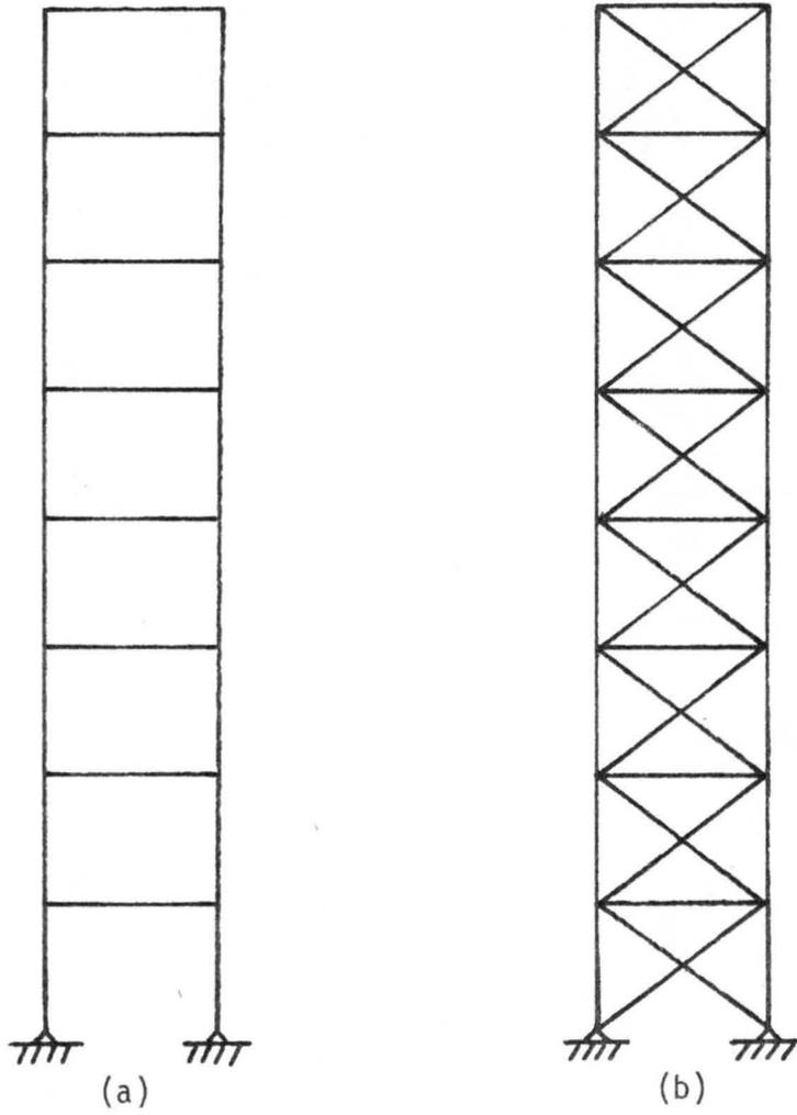
Fig. 3.1 Type 2 frames, laterally unstable (a), and a laterally stable X-braced frame (b).
