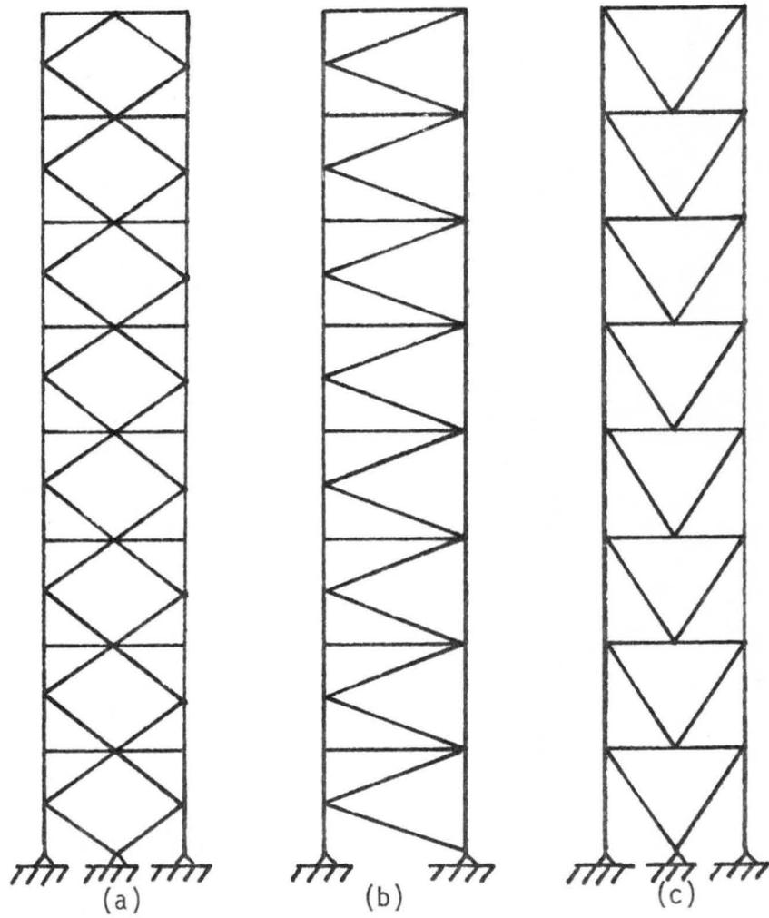
Fig. 3.6 Alternate bracing configurations, diamond bracing (a), K-bracing (b), and V-bracing (c).
