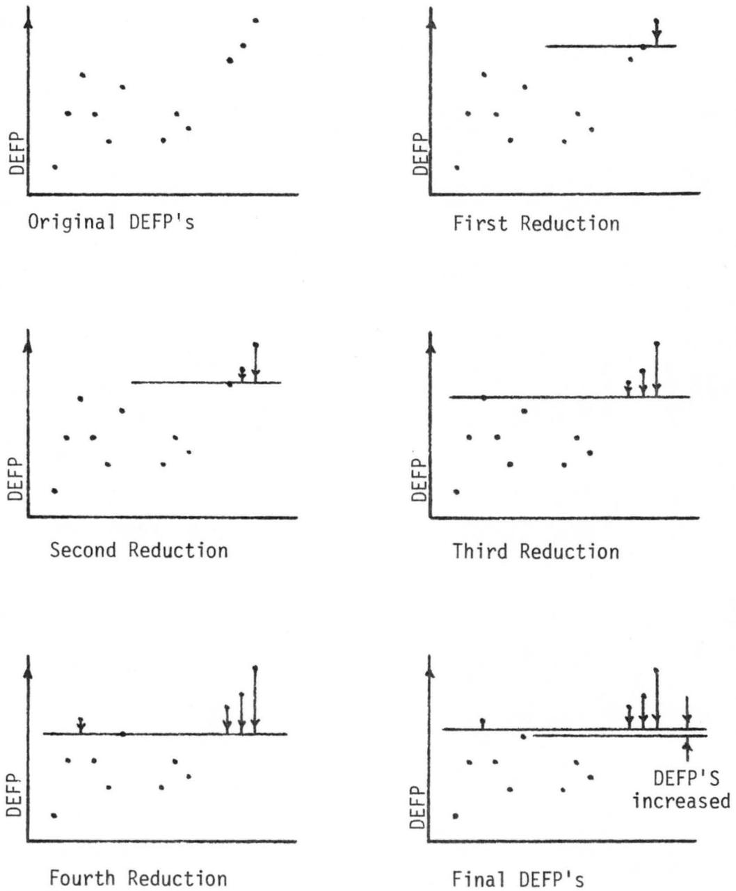
Fig. 4.2 Optimization procedure using the deflection influence parameters.
