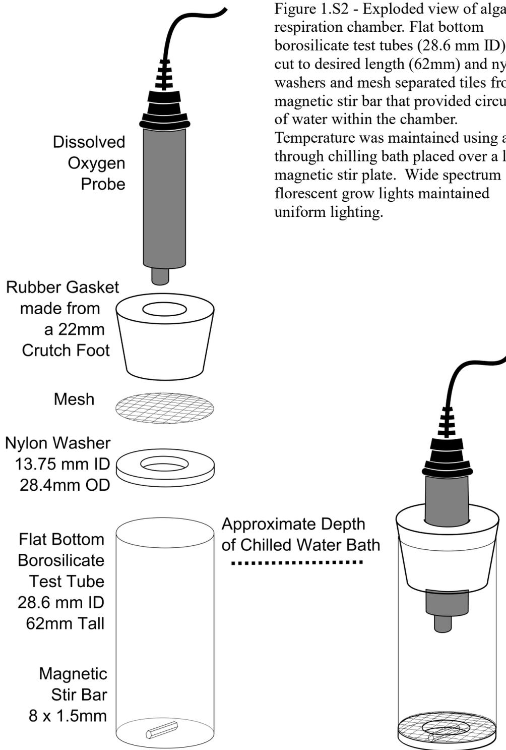
Figure 1.S2 - Exploded view of algal tile respiration chamber. Flat bottom borosilicate test tubes (28.6 mm ID) were cut to desired length (62mm) and nylon washers and mesh separated tiles from a magnetic stir bar that provided circulation of water within the chamber. Temperature was maintained using a flow through chilling bath placed over a large magnetic stir plate. Wide spectrum florescent grow lights maintained uniform lighting.
