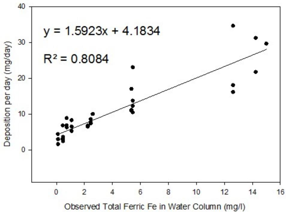
Figure 2.S1 - Deposition of Fe precipitates in Bead Samplers. A: Deposition in bead samplers after only 4 days. Interstitial space was lost in highest 3 treatment levels. B: Dry mass of Fe precipitates (mg/day) was well correlated with Fe observed in the water column ( $R^2=0.8084$ ).
