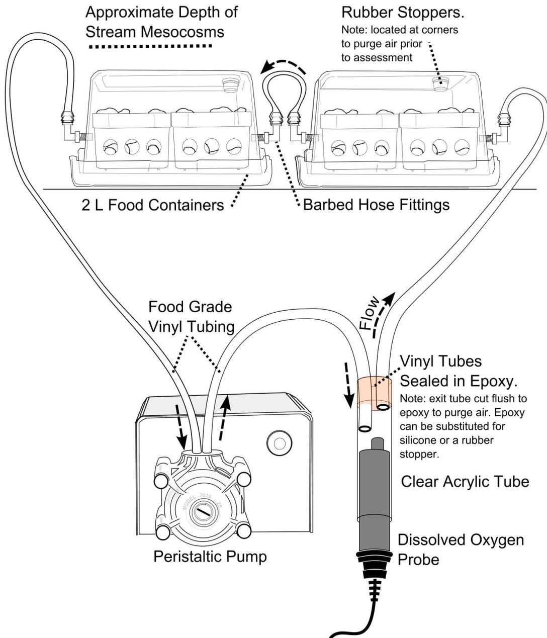
Figure 1.S1 - Schematic of community metabolism chambers. Trays were placed in sealed food containers which were purged of air bubbles. Peristaltic pumps circulated water within the containers through vinyl tubes over a dissolved oxygen probe (YSI Incorporated, Yellow Springs, OH, USA). The tubing and probe were insulated with foam pipe insulation. Dark conditions were created by blocking natural sunlight with opaque black plastic sheeting.
