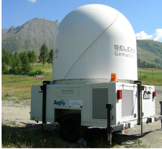
Figure 2.7: X-band mobile radar owned and managed by Arpa Piemonte, during the measurement campaign in the Alps. From Arpa Piemonte.
