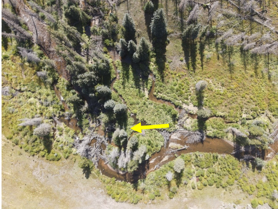
Figure 14: Complex wood accumulations and secondary channels on the South Fork Poudre River restoration at Lazy D Ranch. Flow direction denoted with yellow arrow. (Photo credit: Larimer Conservation District). Photo taken September 2024.
