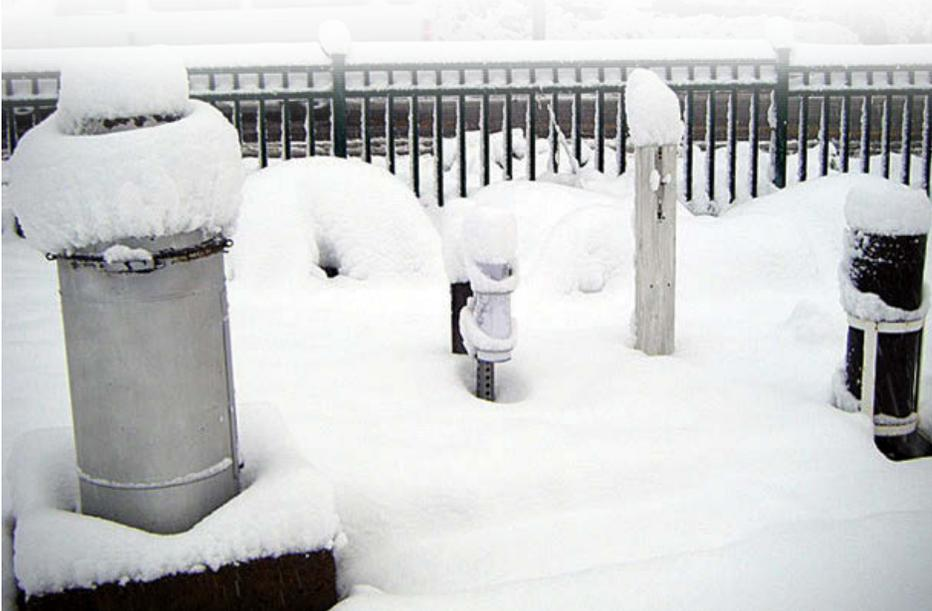
Figure 1. Most precipitation gauges do not measure snow very accurately.
