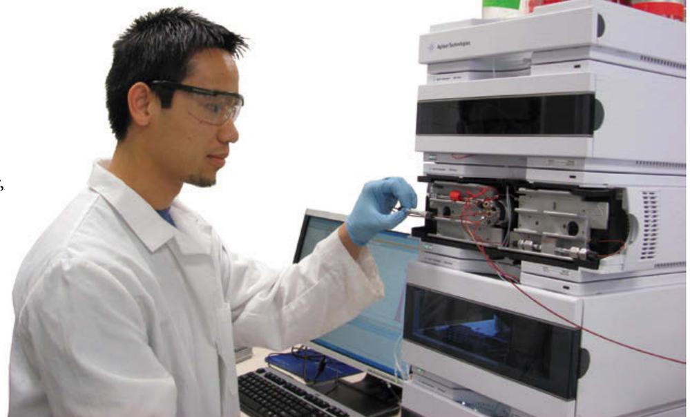
*Victor Sam sets up the HPLC (High Performance Liquid Chromatography) for microcystin-LR analysis. GC & LC/MS/MS analysis was done at the Center for Environmental Medicine Analytical Lab at Colorado State University.*
