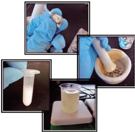
*Extraction procedure of active component of the moringa oleifera tree seed. Steps involved deshelling, pulverization, salting and purification. Extraction and experimental procedures performed at the Department of Civil & Environmental Engineering Water Quality Lab at Colorado State University.*
