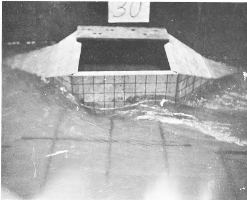
Fig. No. 4-11 Photo of wing-wall abutments
