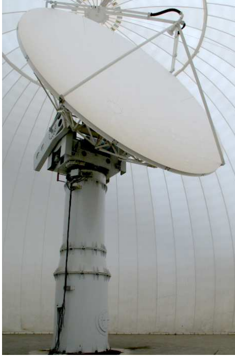
Figure 2.6: The CSU-CHILL antenna and pedestal as it looked until July 2007 and the version used to collect data analyzed in this thesis.
