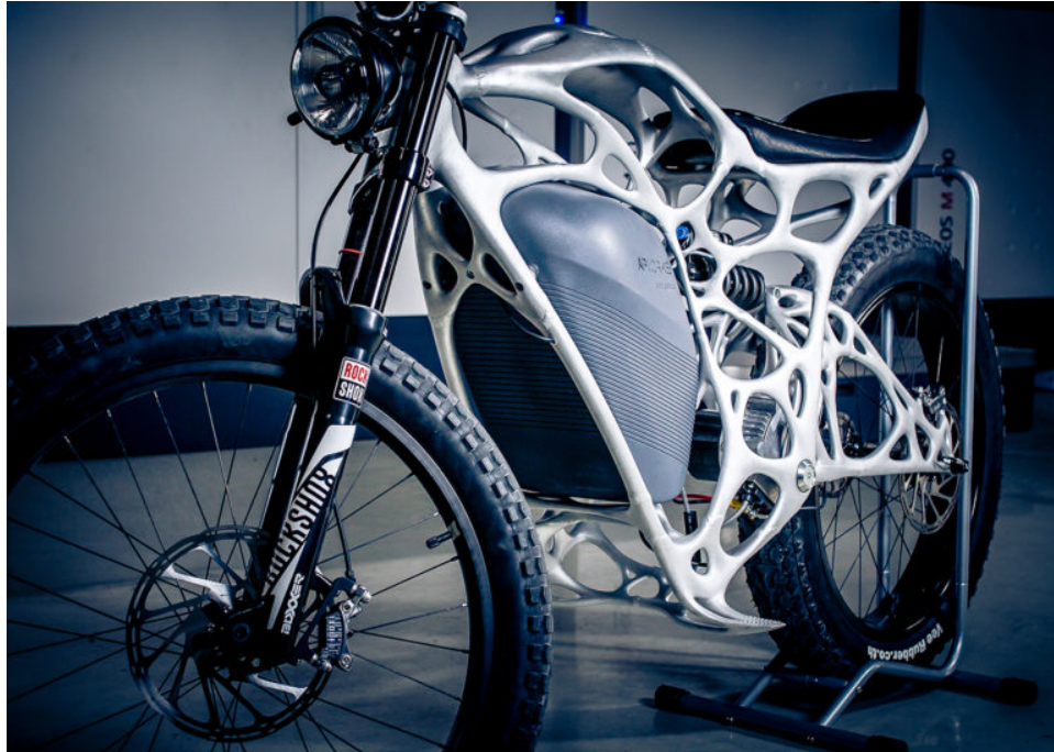
Figure 1.5: A bicycle designed using topology optimization by APWorks and then 3D-printed – image from APWorks.
