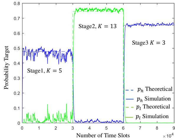
**Figure 5.7:** Entries of transmission probability vector in multi-packet reception channel
