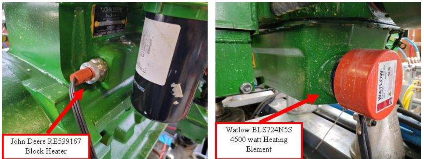
Fig. 8. Right: Block heater placement on rear of engine. Left: Heating element placement in oil pan.
