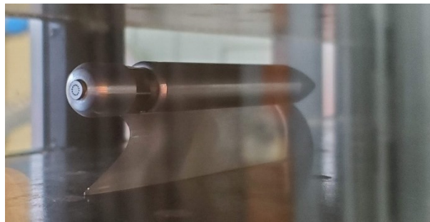
Figure 4.3: Stagnation pressure probe installed in the test section
