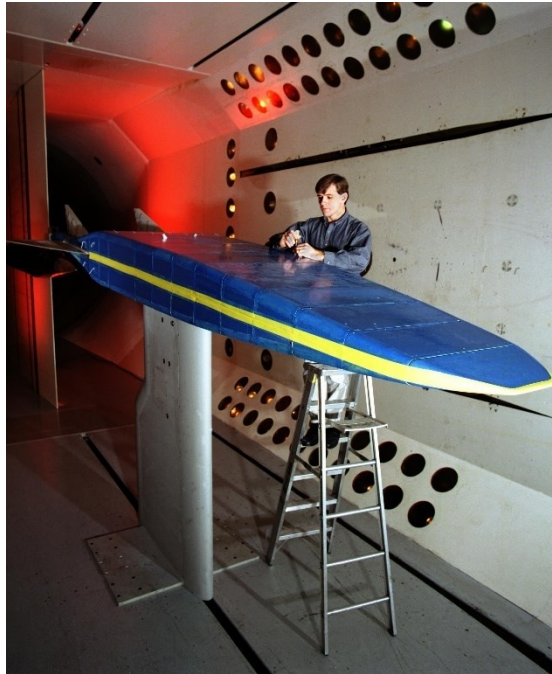
Figure 1.3: National Aero-Space Plane 1/3 scale wind tunnel model [3].
