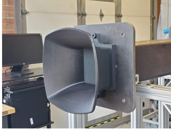
Figure 3.15: Indraft wind tunnel bellmouth atmospheric intake
