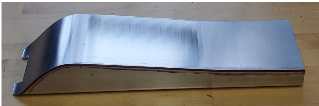
Figure 3.16: Aluminum billet nozzle for Mach 2.5 for 5.25" x 1.7" test size
