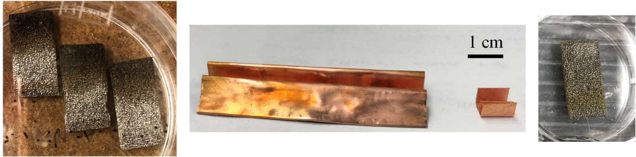
Figure 6.10. Photographs of two sample holders (center); and VGN samples resulting from the larger sample holder (left) and smaller sample holder (right).
