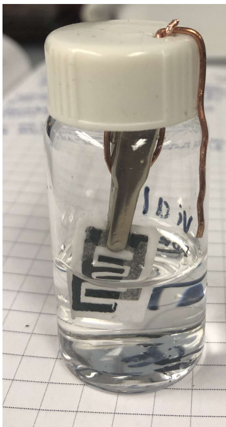
Figure 2.1. Photograph of modified glass scintillation vial used for SnO 2 TF growth on a paper substrate with printed electrodes.
