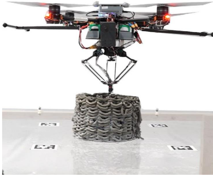
Figure 1-8: Cementitious, cylindrical print demonstrating the capabilities of aerial additive manufacturing [31].
