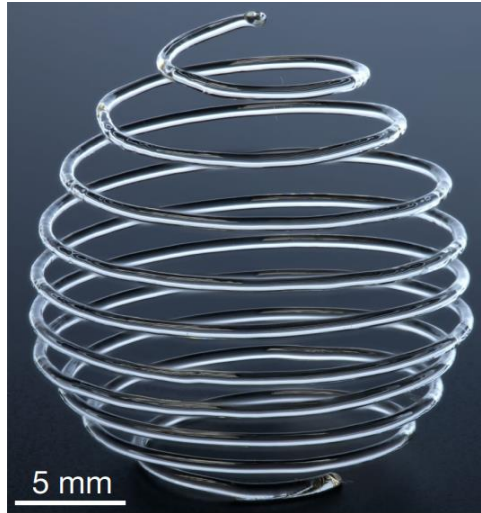
Figure 1-4: Complex, free-form 3D printed structure manufactured using frontal polymerization [11].
