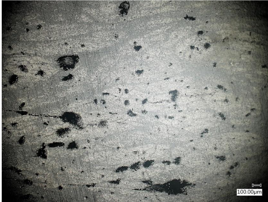
Figure 3-7: Cross-sectional micrograph of the 6.1 mm thick composite part.
