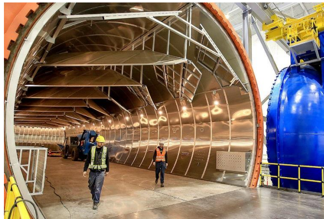
Figure 1-1: Industrial autoclave used to manufacture airplane wings for Boeing [9].
