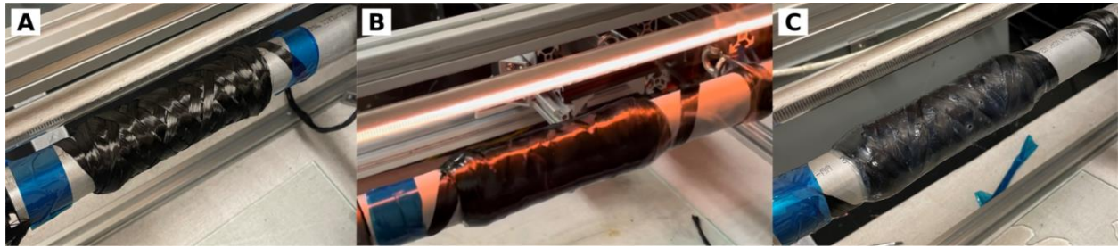
Figure 3-5: First part wound using the redesigned filament winder machine where A) is the dry fiber test run, B) is the wet wound part after the IR bulb is powered on, and C) is the cured part.
