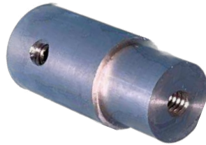
Figure 2-2: Custom machined wheel hubs to adapt stepper motors to mecanum wheels.
