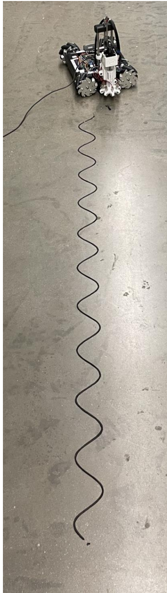
Figure 2-53: 2.5 m long sin wave printed on concrete floor to demonstrate part size capabilities.
