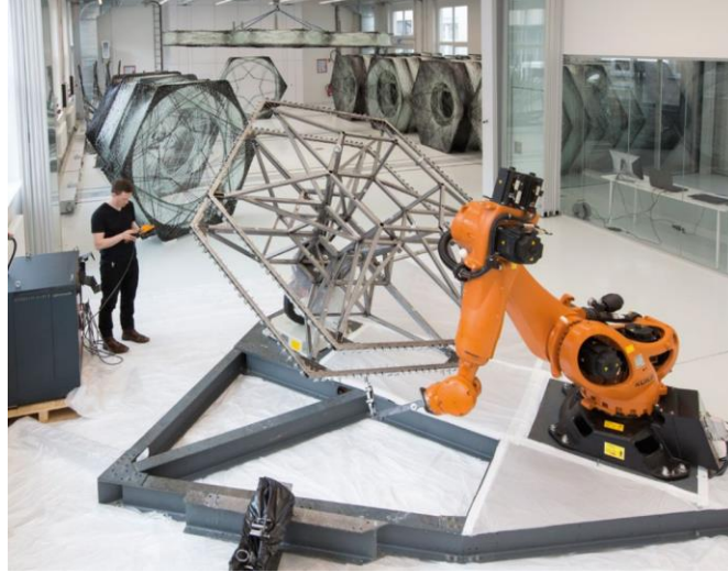
Figure 1-15: Researchers at the University of Stuttgart using a complex filament winding machine for winding of structural, fiber-reinforced composite parts [40].
