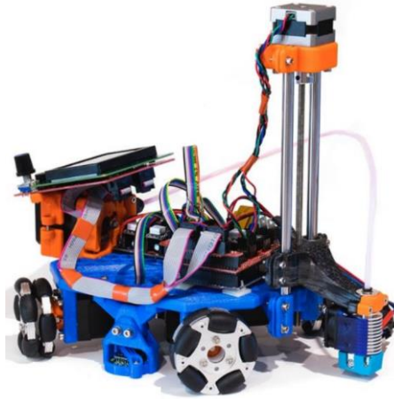
Figure 1-9: Simple, low cost robotic platform for MAM [29].
