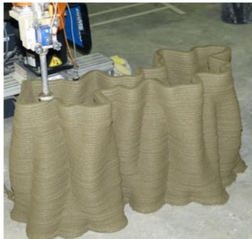
Figure 1-11: Funicular architectural geometry manufacturing using a holonomic platform [35].
