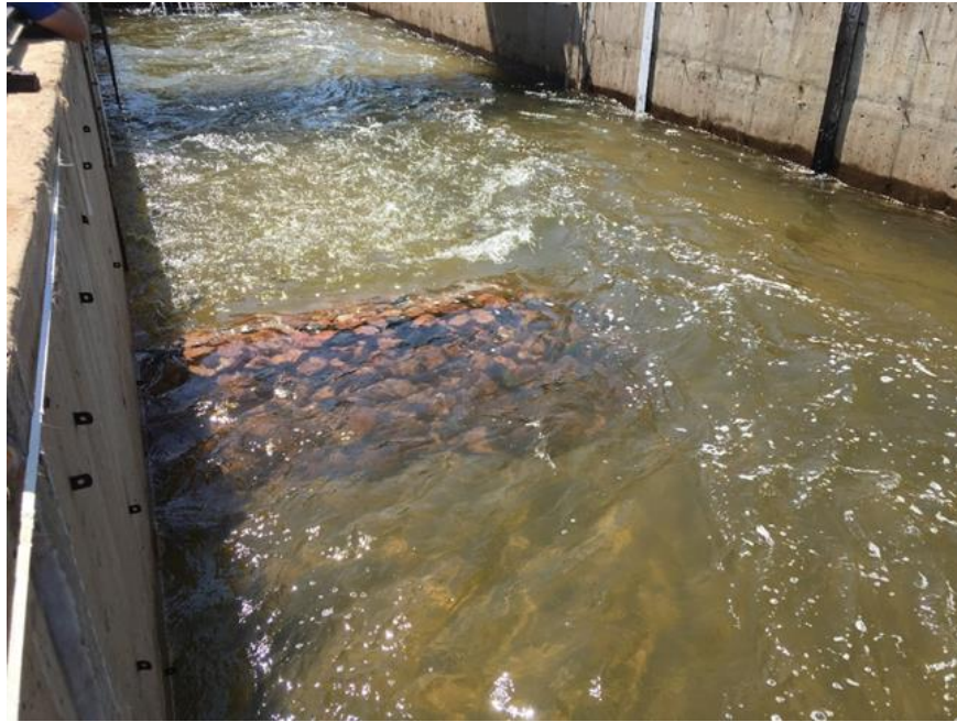
Figure 2: A view of the single bendway weir formed in the sediment recess of CSU's large (20.0 ft wide, 8.0 ft deep) flume located outdoors. In this experiment, y/H = 1.25
