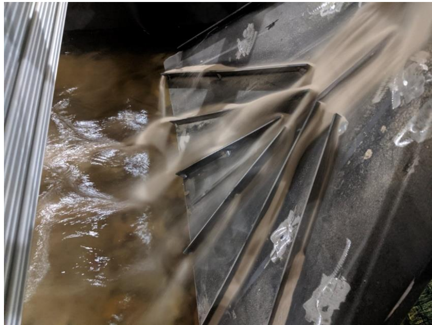
Figure 29: Sediment diffuser located at the base of the sand-feed hopper
