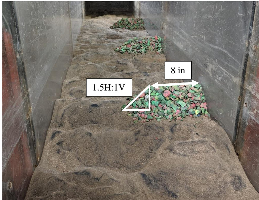
Figure 13: Side profile of a BW placed in the 2ft flume
