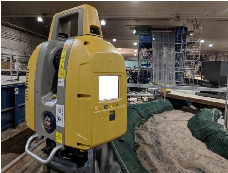
Figure 32: A LiDAR instrument scanned the channel bed after a completed experiment
