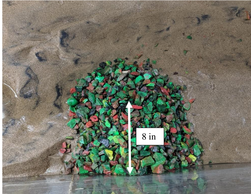
Figure 16: Plan profile of a RV placed in the 2 ft flume
