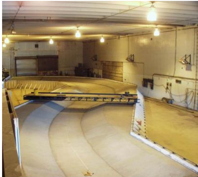
Figure 1: CSU's hydraulic model of a reach of the Middle Rio Grande River (Scurlock et al. 2014)
