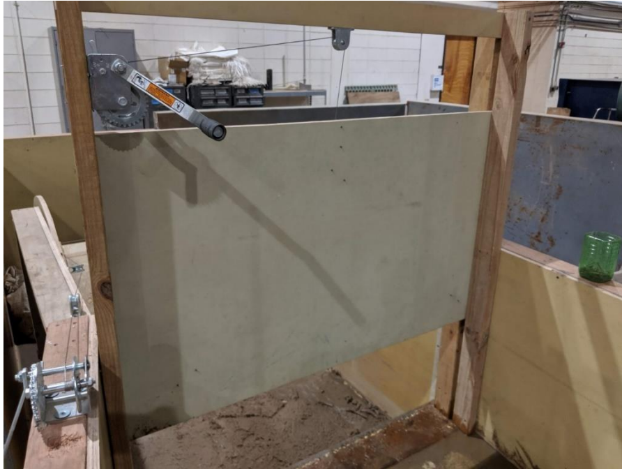
Figure 24: The vertical sluice gate used for the curved flume
