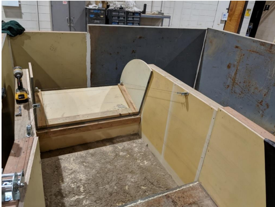
Figure 25: The overshot gate (or sloped weir) used for the curved flume. The gate is positioned immediately downstream of the flume's tailbox.
