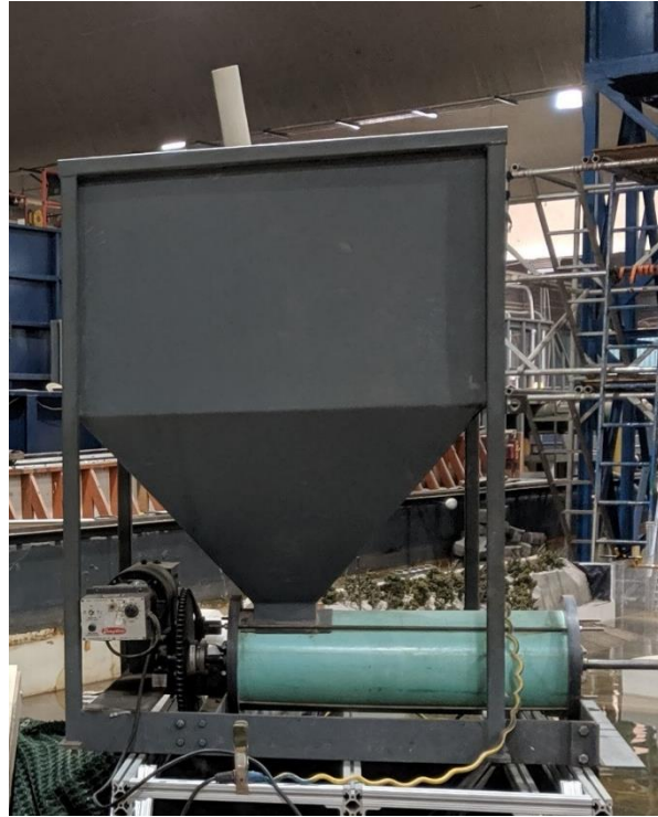
Figure 28: The sediment hopper used to feed sand into the approach to the curved flume
