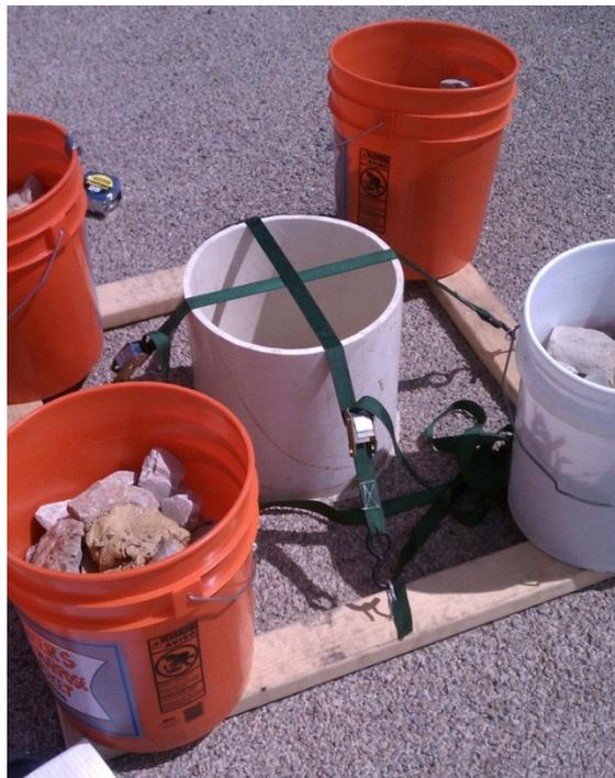
**Figure 16: Infiltration test setup at CTL on 5/03/2012**
