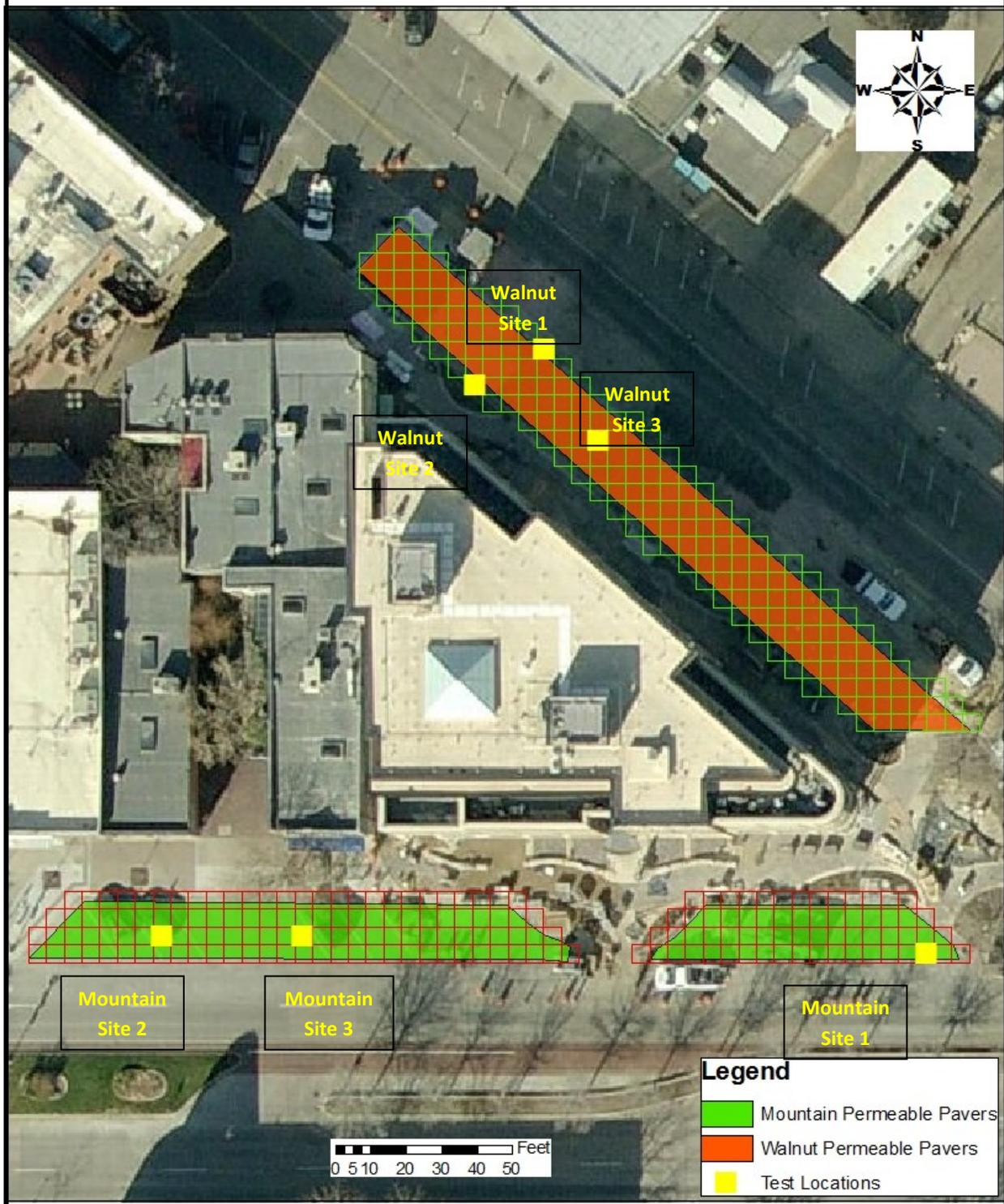
Figure 17: Infiltration test locations at the Mitchell Block sites
