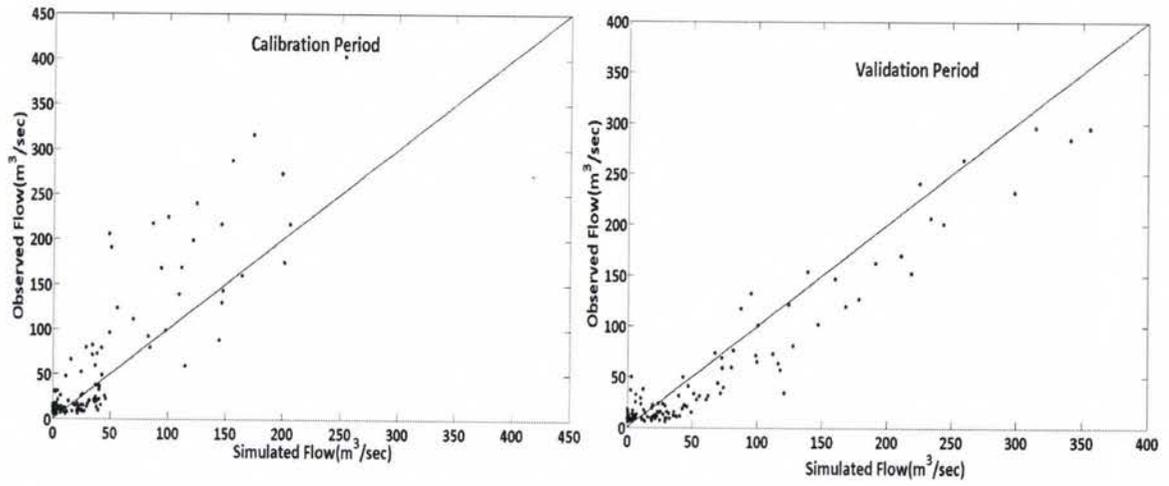
Figure A2.5. Scatter plot between the observed and simulated flows during the calibration and validation period for Yampa River basin
