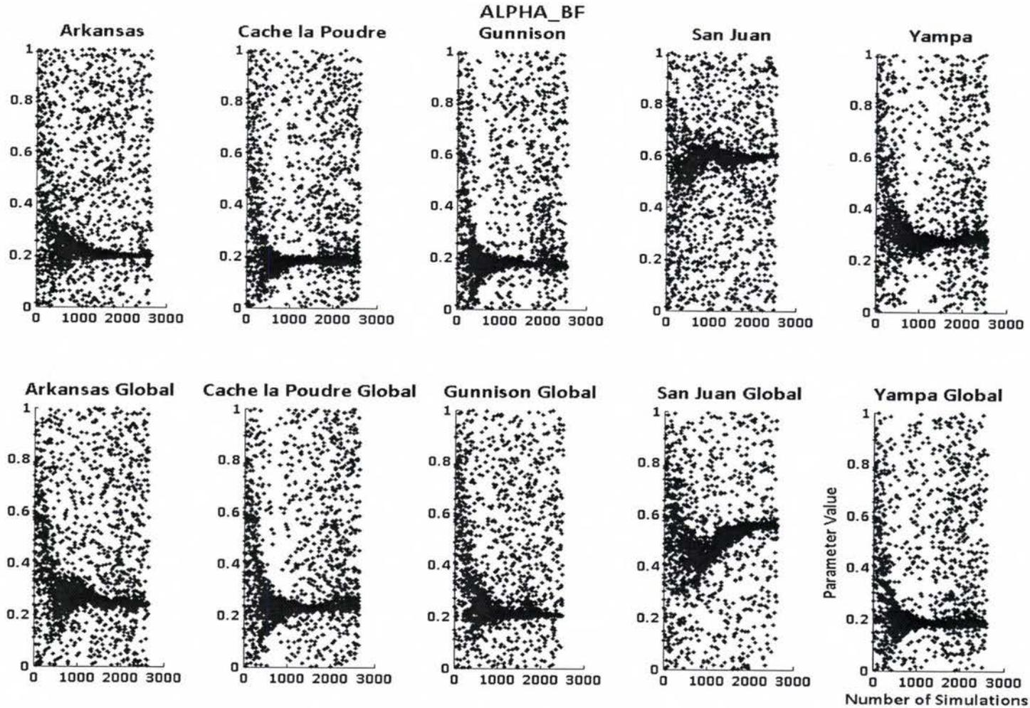
Figure A2.6. Convergence of parameter value for ALPHA\_BF from single-site and multi-site calibration of SWAT model for the study
