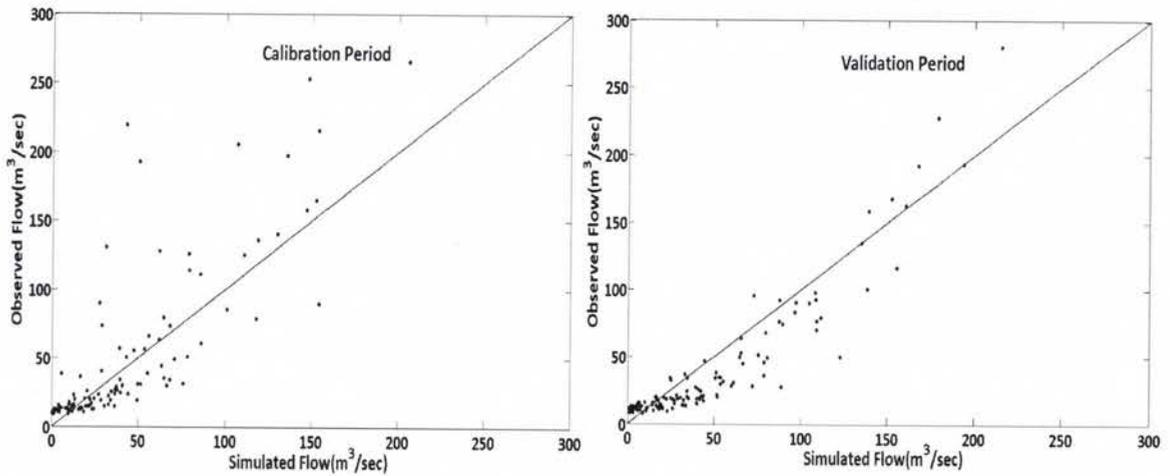
Figure A2.3. Scatter plot between the observed and simulated flows during the calibration and validation period for Gunnison River basin
