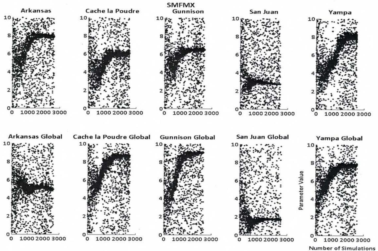
Figure A2.11. Convergence of parameter value for SMFMX from single-site and multi-site calibration of SWAT model for the study
