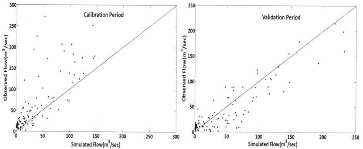
Figure A2.4. Scatter plot between the observed and simulated flows during the calibration and validation period for San Juan River basin
