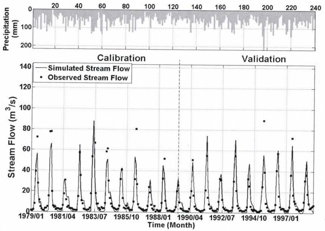
Figure 3.4. Measured and simulated total monthly streamflow for calibration and validation period from the single-site calibration of SWAT model for Cache la Poudre River basin
