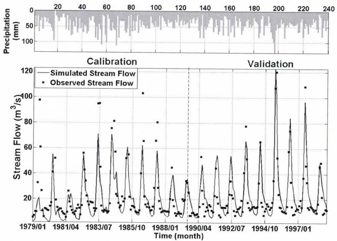
Figure 3.3. Measured and simulated total monthly streamflow for calibration and validation period from the single-site calibration of SWAT model for Arkansas River basin.
