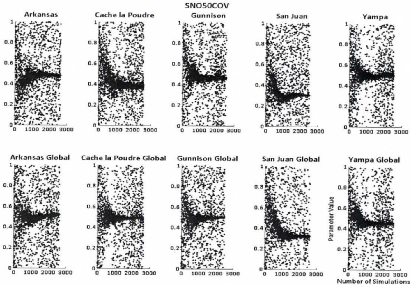
Figure A2.12. Convergence of parameter value for SNO50COV from single-site and multi-site calibration of SWAT model for the study
