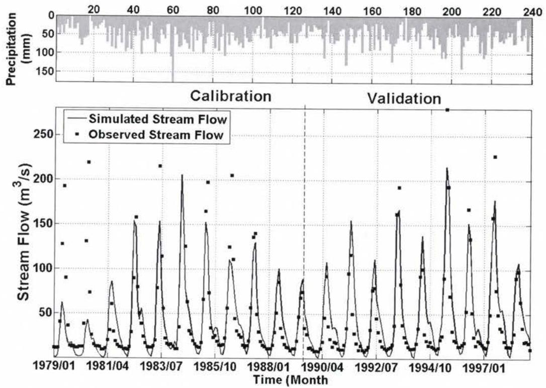
Figure 3.5. Measured and simulated total monthly streamflow for calibration and validation period from the single-site calibration of SWAT model for Gunnison River basin.
