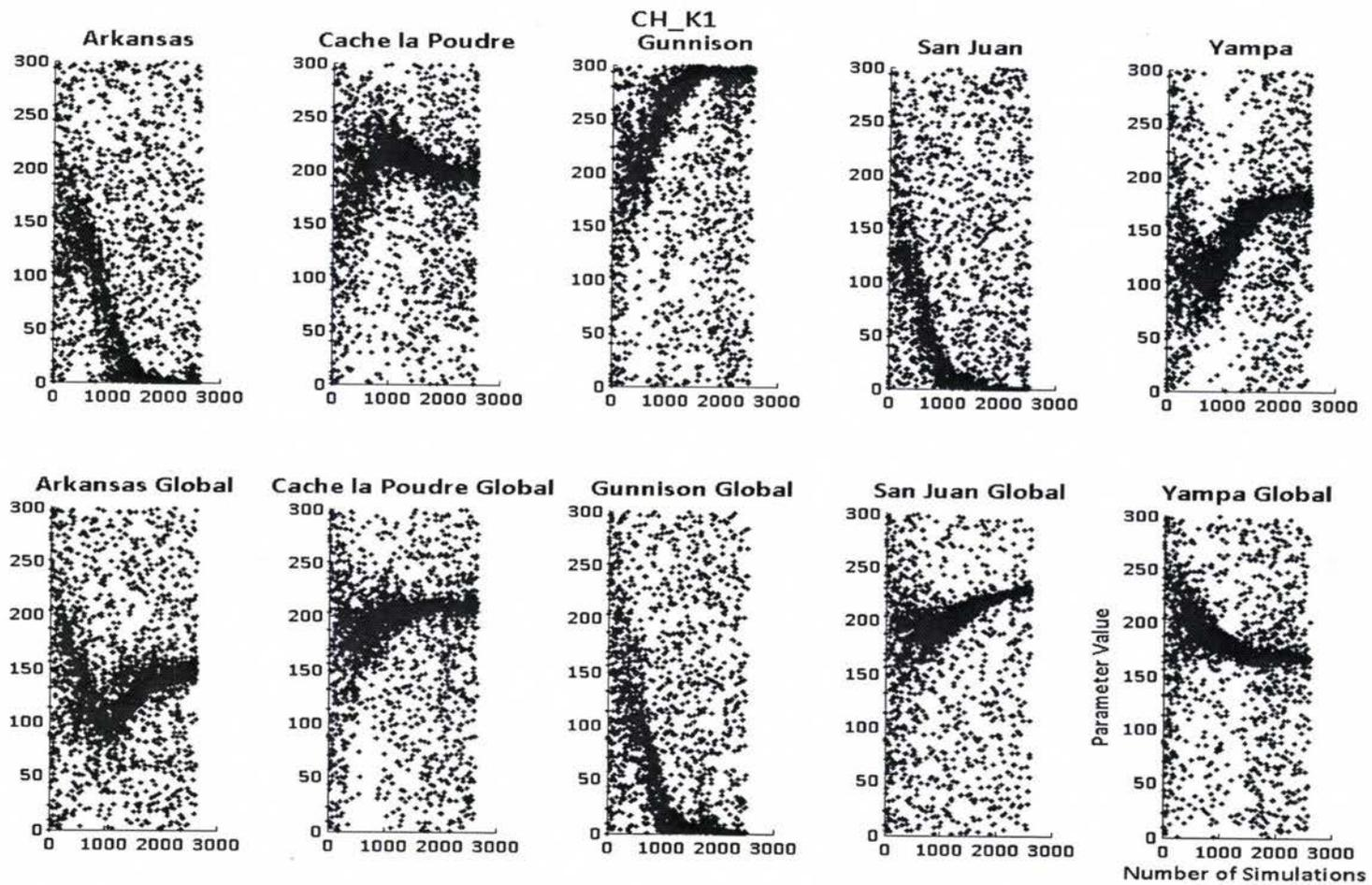
Figure A2.7. Convergence of parameter value for CH\_K1 from single-site and multi-site calibration of SWAT model for the study watersheds.
