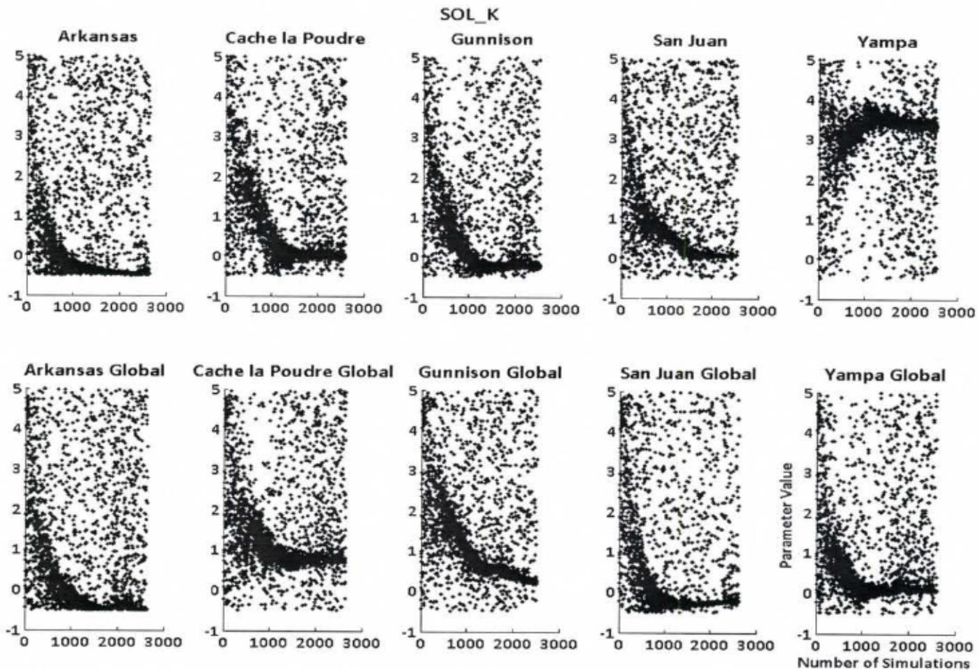
Figure A2.15. Convergence of parameter value for SOL\_K from single-site and multi-site calibration of SWAT model for the study watersheds.
