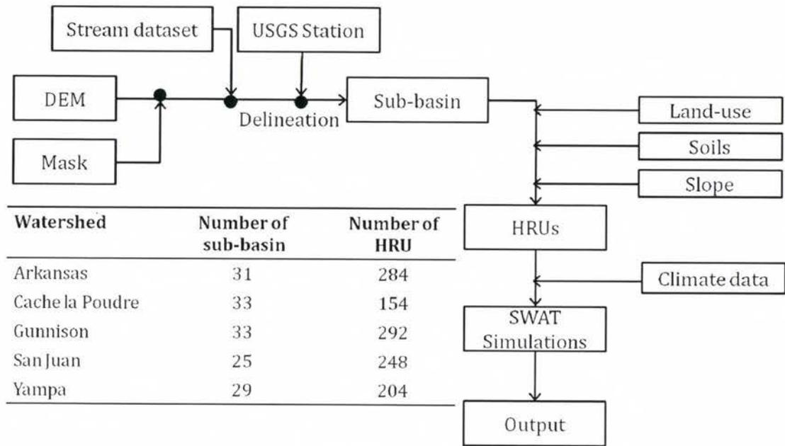
Figure 2.8. Schematic of SWAT project set up
