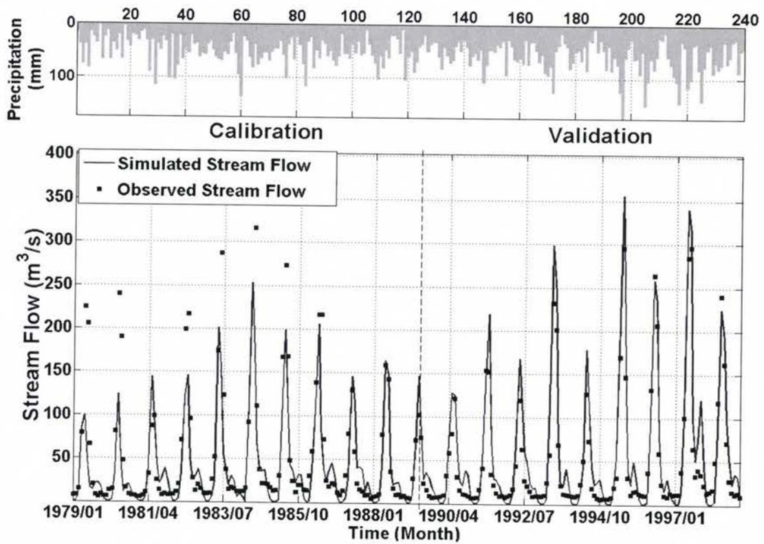
Figure 3.7. Measured and simulated total monthly streamflow for calibration and validation period from the single-site calibration of SWAT model for Yampa River basin.
