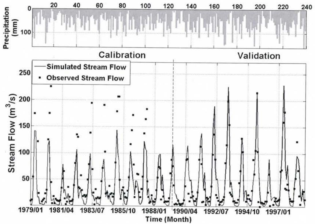
Figure 3.6. Measured and simulated total monthly streamflow for calibration and validation period from the single site calibration of SWAT model for San Juan River basin.
