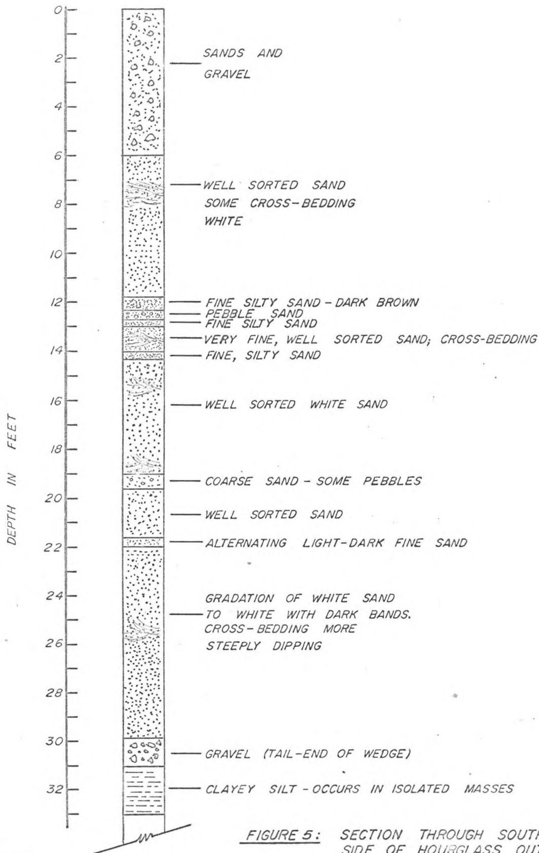
**FIGURE 5:** SECTION THROUGH SOUTH SIDE OF HOURGLASS OUTLET.
