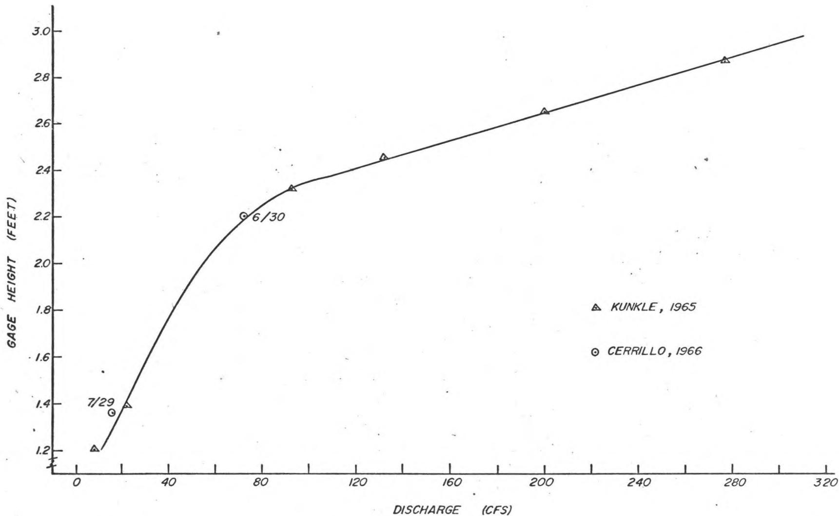
FIGURE 12. STAGE-DISCHARGE CURVE, SECTION 2 (AFTER KUNKLE, 1967)
