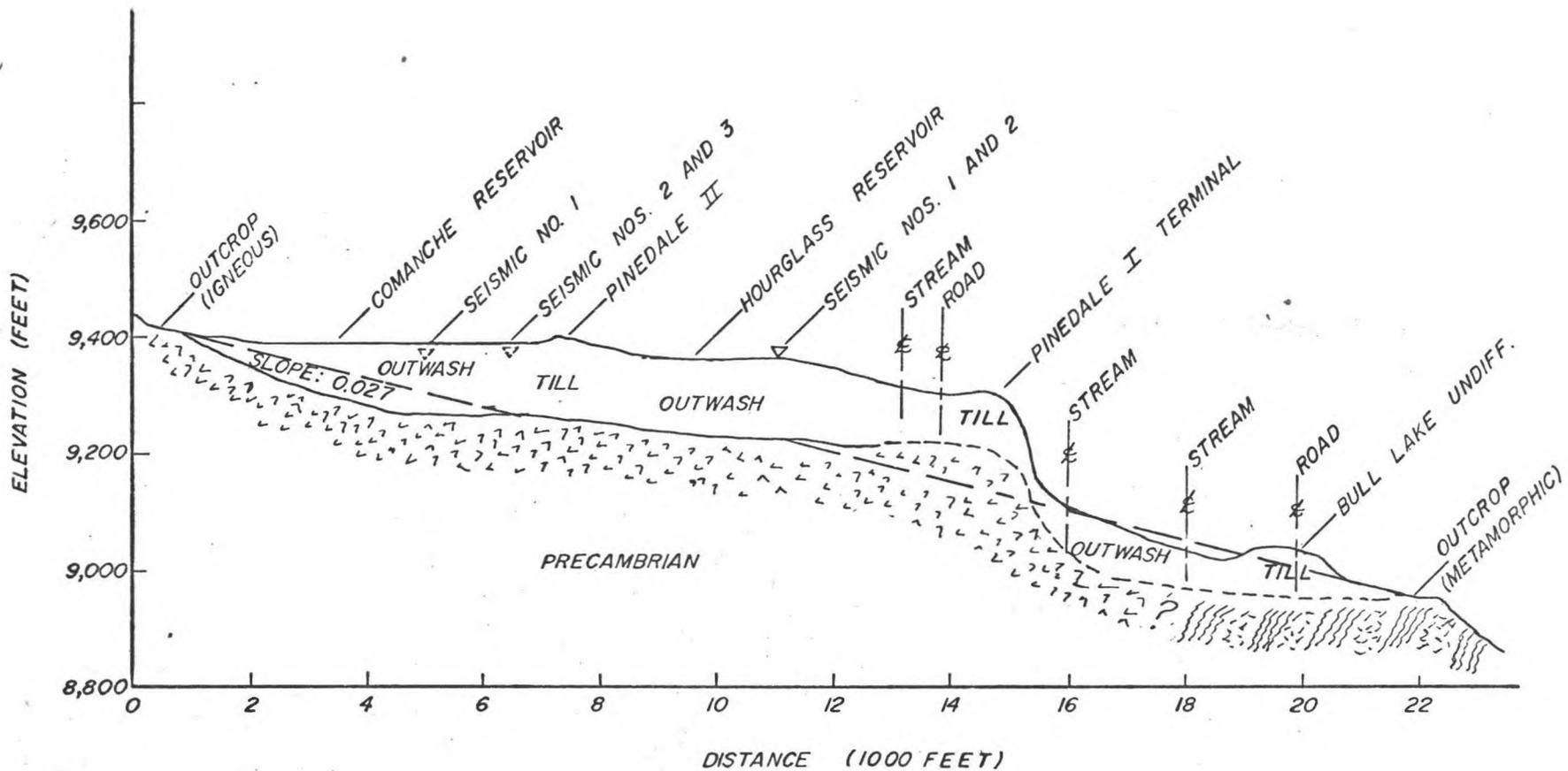
FIGURE 10: SECTION ALONG AXIS OF MAIN BASIN (SEE FIG. 1 FOR LOCATION)
