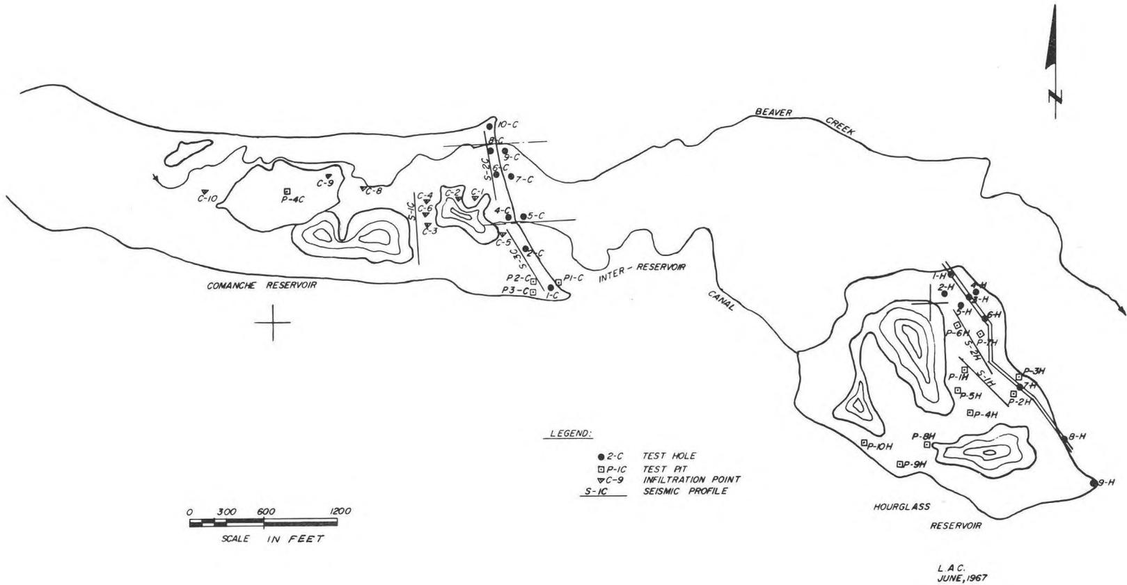
FIGURE 9: TEST HOLE, SEISMIC AND INFILTRATION LOCATION MAP.
