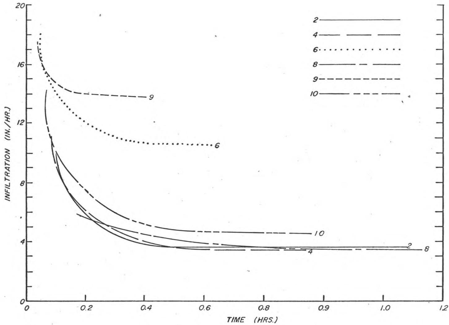
FIGURE 8: INFILTRATION RATES WITHIN COMANCHE RESERVOIR.
