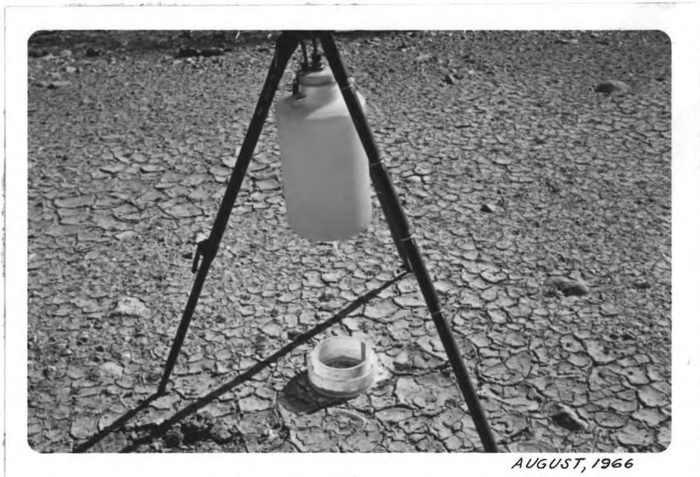
Plate 1.--Double-ring infiltration apparatus with mariotte feed bottle.
