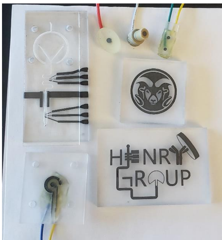
Figure 3.1 Image of PCL TPEs pressed in various templates with different shapes and designs.
