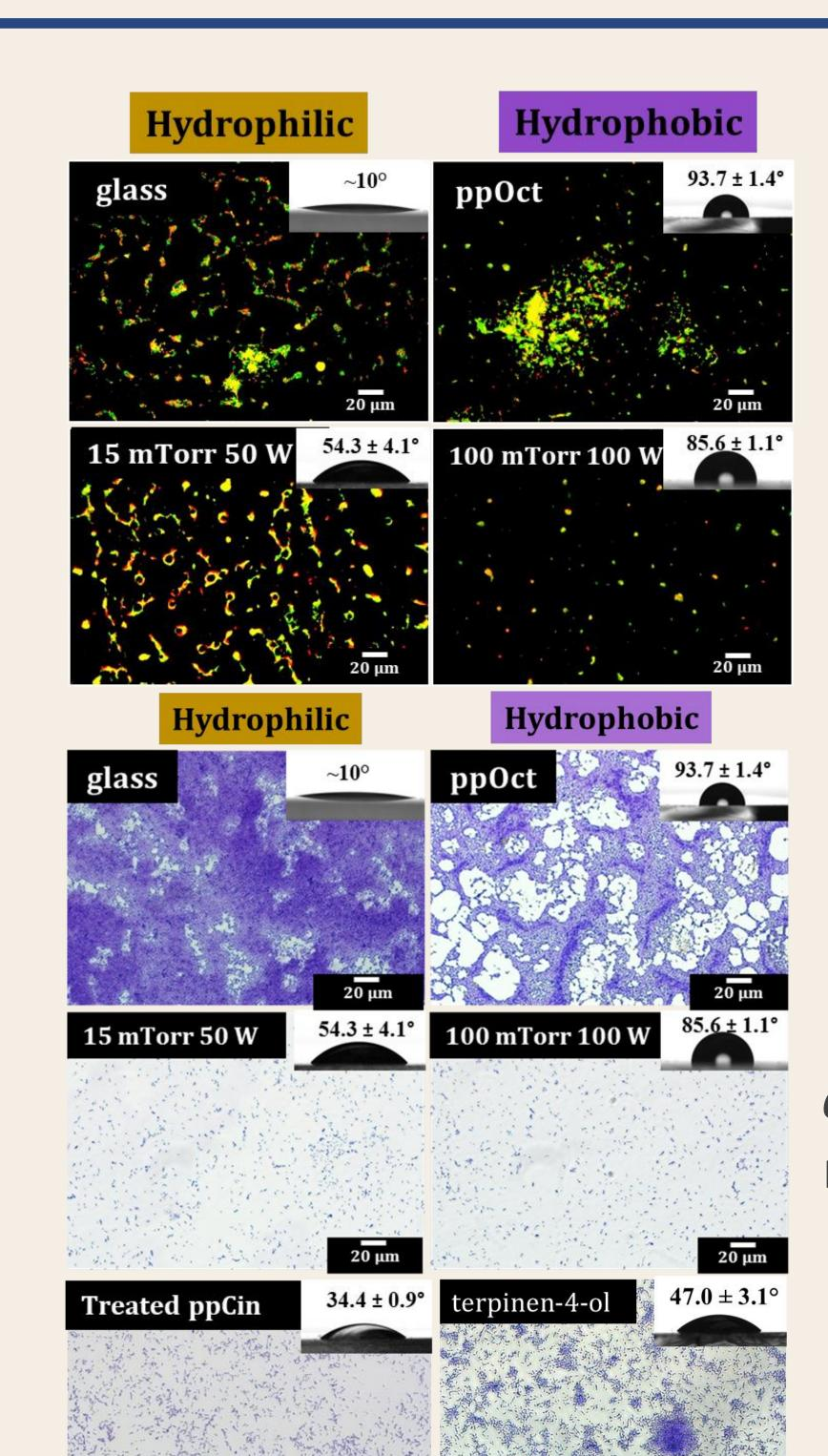
When deposited on filtration membranes, coatings resist protein adsorption and maintain performance of membranes, making them ideal for blood dialysis and water treatment.
