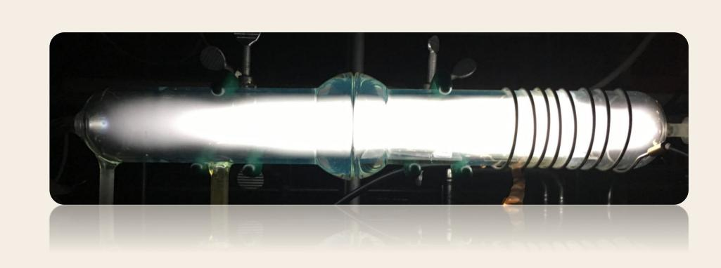
In <u>PECVD</u>, the essential oil serves as a liquid monomer and is introduced to the plasma reactor chamber where reactive species are generated. These reactive essential oil species polymerize to <u>conformally coat the biomaterial</u> with an adherent pinhole-free thin film.
