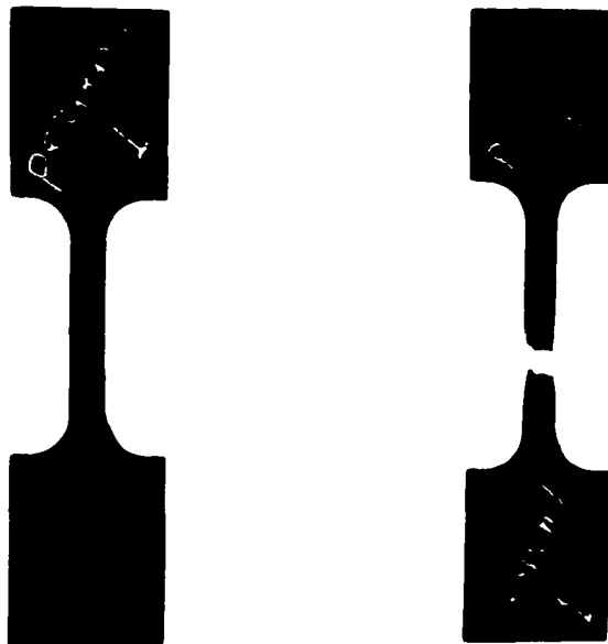
Figure 3.2.2.4 Web samples of HPS70W for uniaxial tensile tests - Perpendicular to rolling direction
