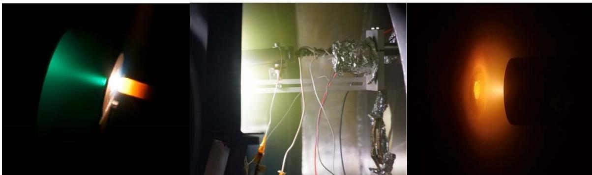
*Figure 4.1: Photographs of cathodes operating on iodine at all three facilities: UA (left), MSFC (middle), CSU (right).*
