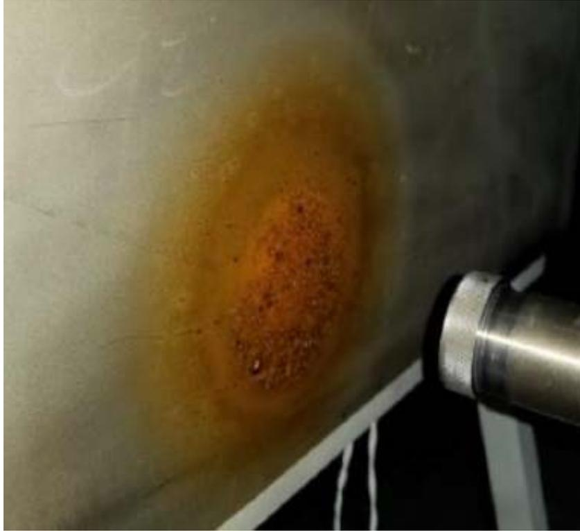
*Figure 4.3: Iodide containing film on stainless steel anode after 8.4 four test conducted at MSFC. Film buildup over time believed to cause anode voltage to change.*
