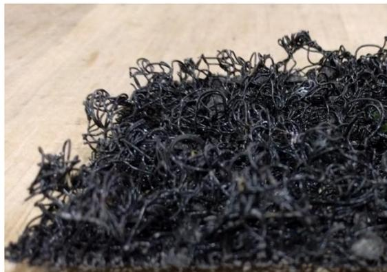
Figure 19. Detail of non-woven monofilament geo-net composite material.
