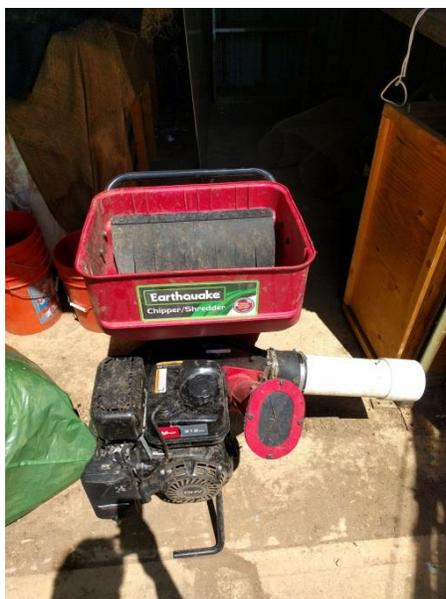
Figure 31: Waste shredder with 4” PVC nozzle installed on the outlet
