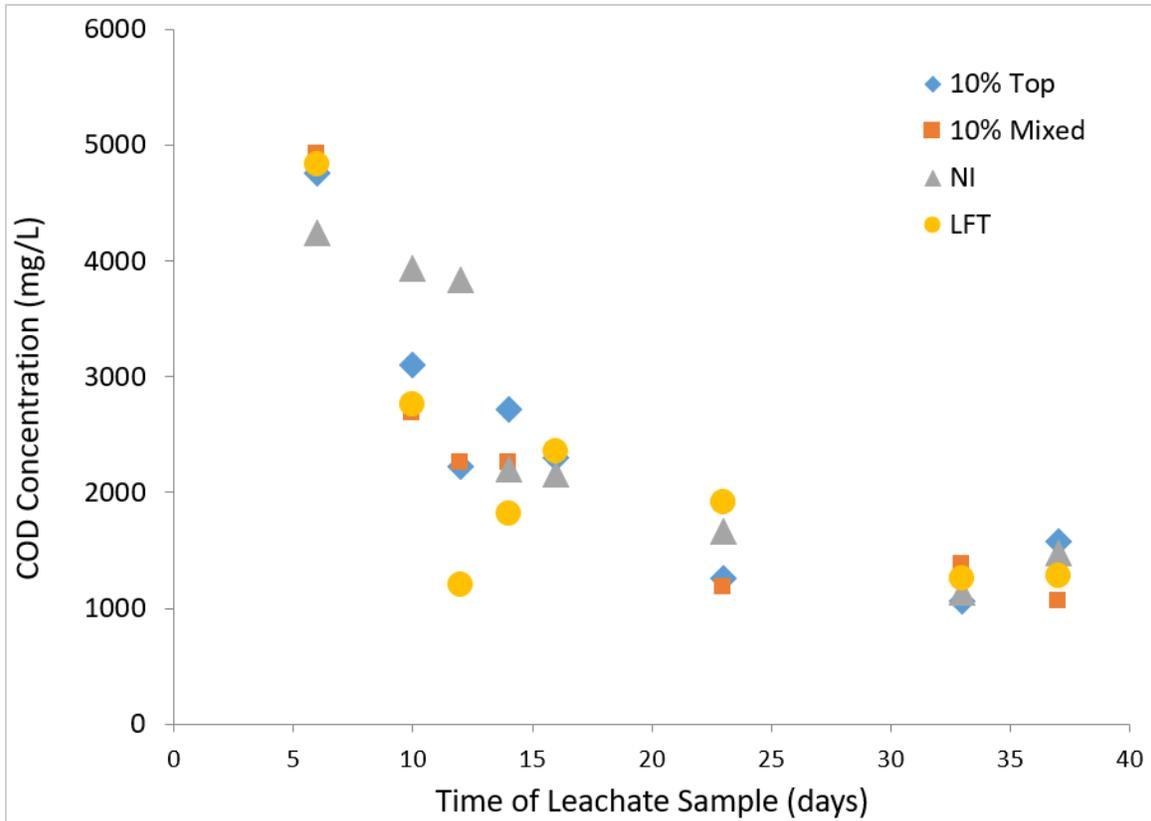
Figure 34: COD of the Leachate at the Exit of the 3 LBRs and the LFT Tank.
