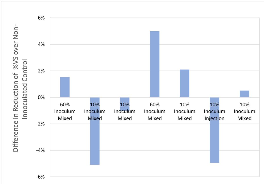
Figure 32: Experimental batches 1-4 with the Percent Improvement for VS Destruction of the Inoculated Batches versus Non-Inoculated Control for that Batch of Experiments
