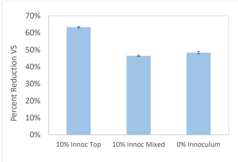
Figure 33: Percent Reduction VS during Digestion Process (error bars represent replicates of analytical samples of VS taken from the same sample)
