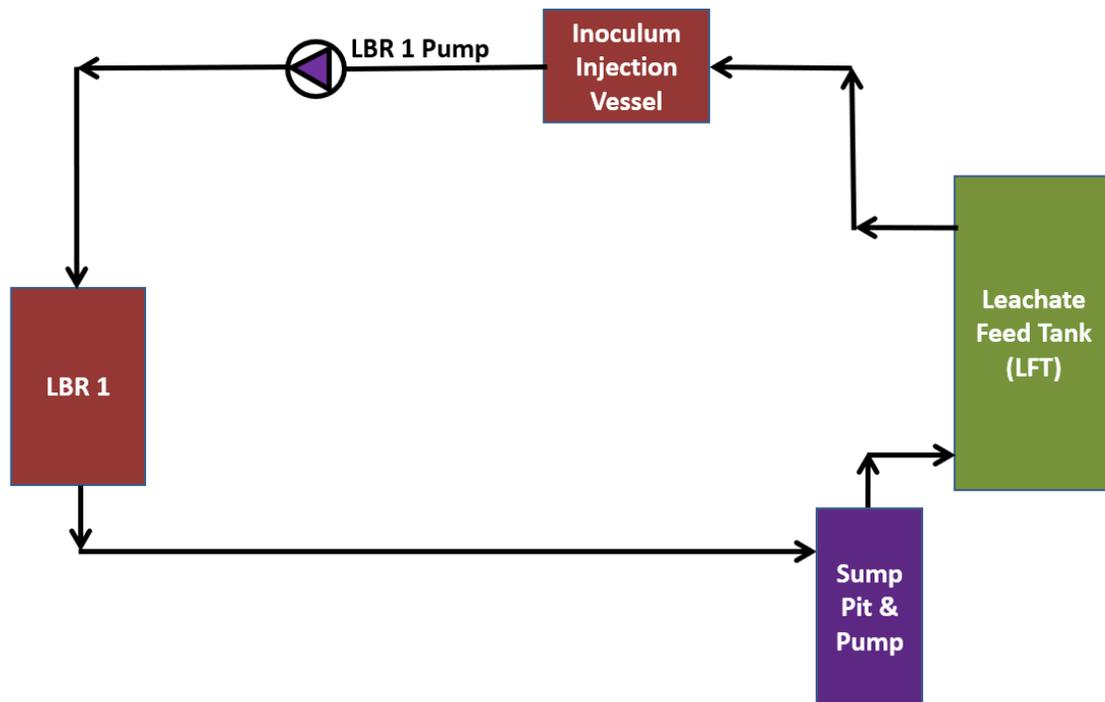
Figure 29. Inoculum injection process diagram
