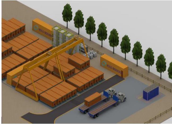
Figure 6: Rendering of possible layout for commercial scale MSAD system using LBR modules
