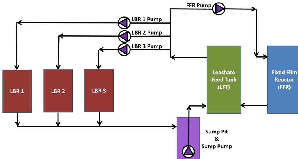
Figure 9: Process Diagram of MSAD Demonstration-Scale System
