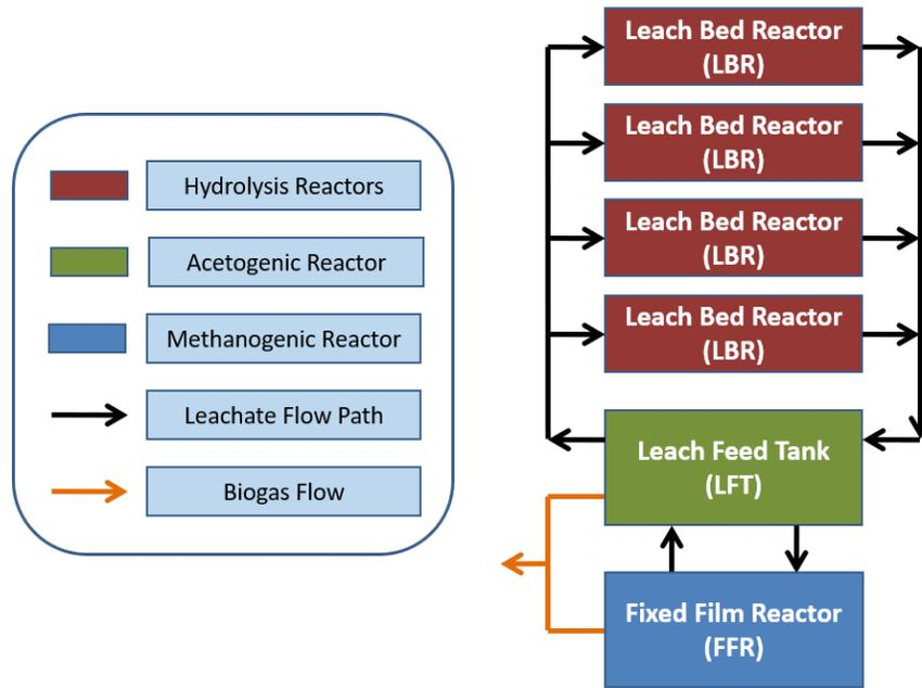
Figure 5: The CSU Multistage Anaerobic Digestion Process Flow Diagram
