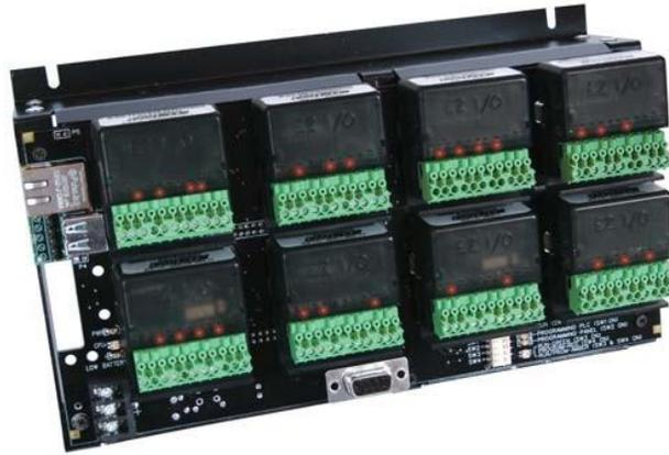
Figure 10. Eight I/O modules plugged into a PLC base
