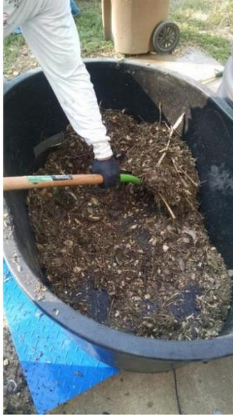
Figure 27. 110 Gallon mixing tank. Note blue pallet scale which is used to measure the substrates mass.
