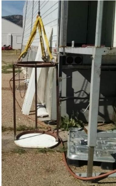
Figure 30. Drum elevator next to loading dock
