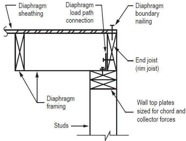
Figure 1.6 Components of a Diaphragm
