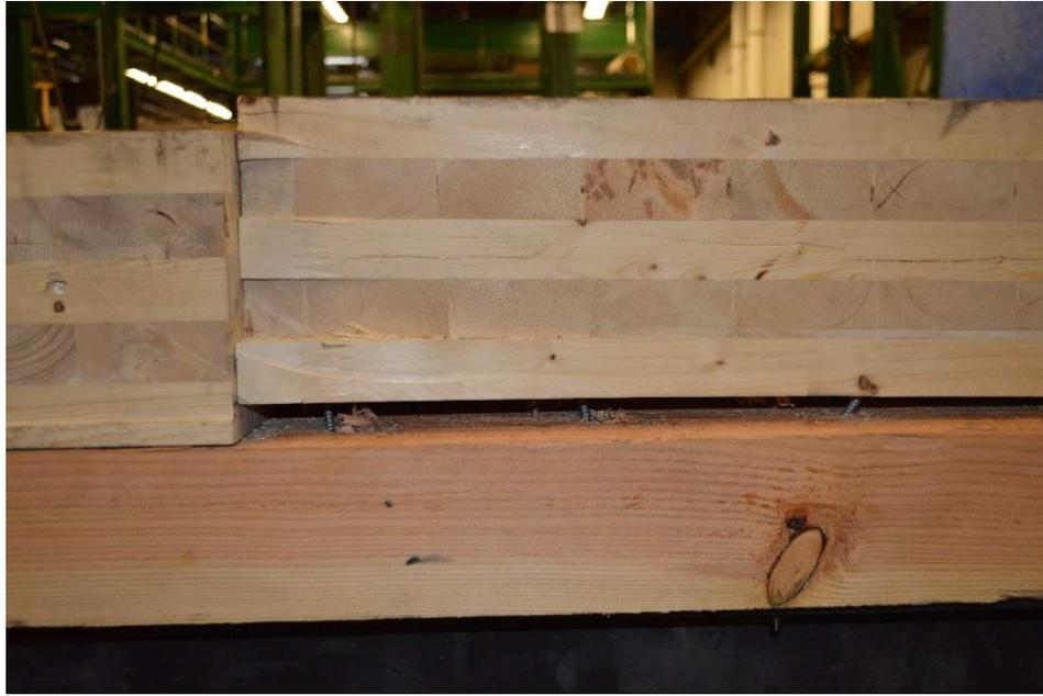
Figure 4.8 SDS screw shear failure
