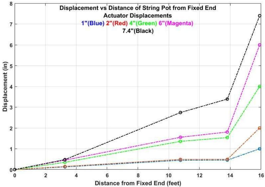
Figure 4.23 Displacement of String Pots vs Distance of String Pots from fixed end
