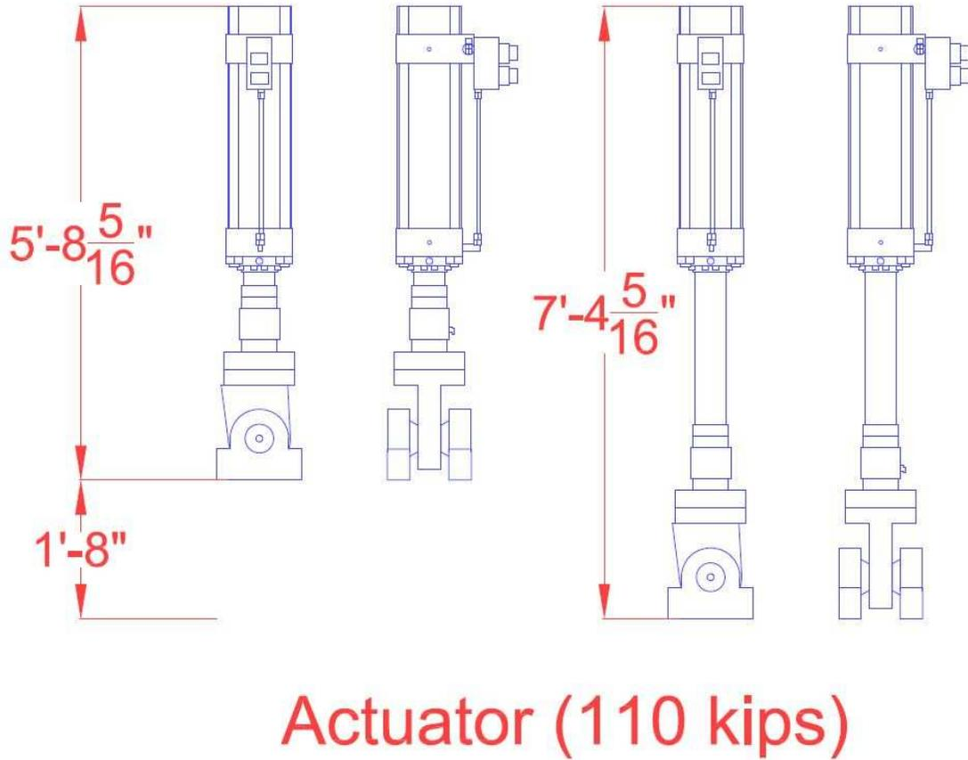
Figure A.1 Actuator Top and Side Views (Fully Compressed and Fully Elongated)
