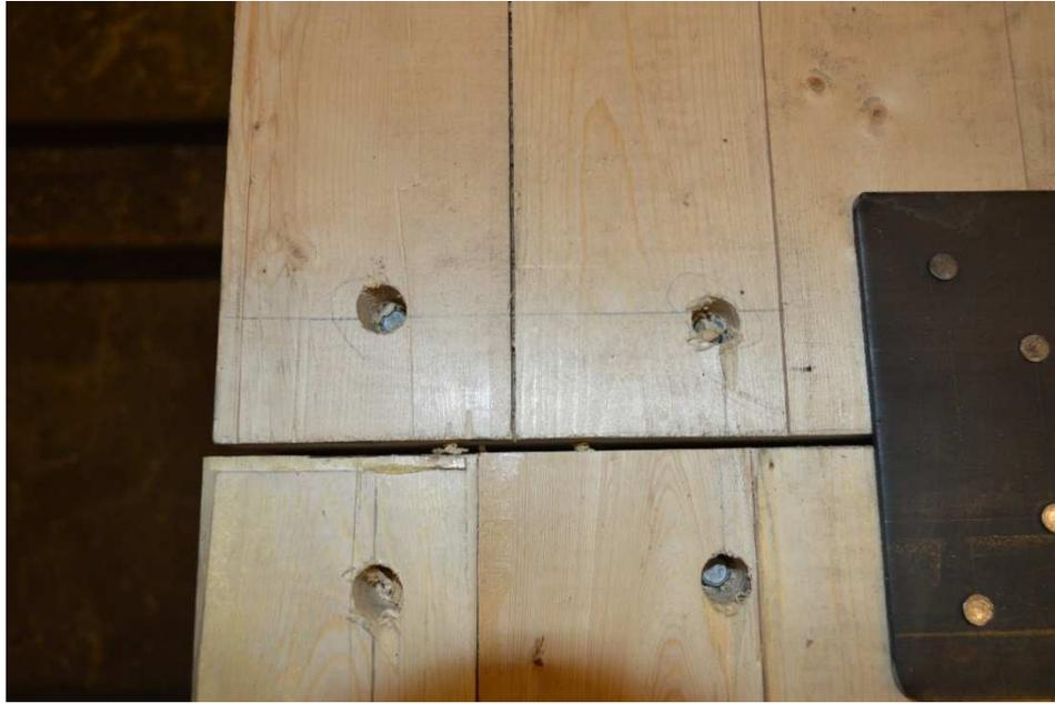
Figure 2.4 SDS Screws into CLT
