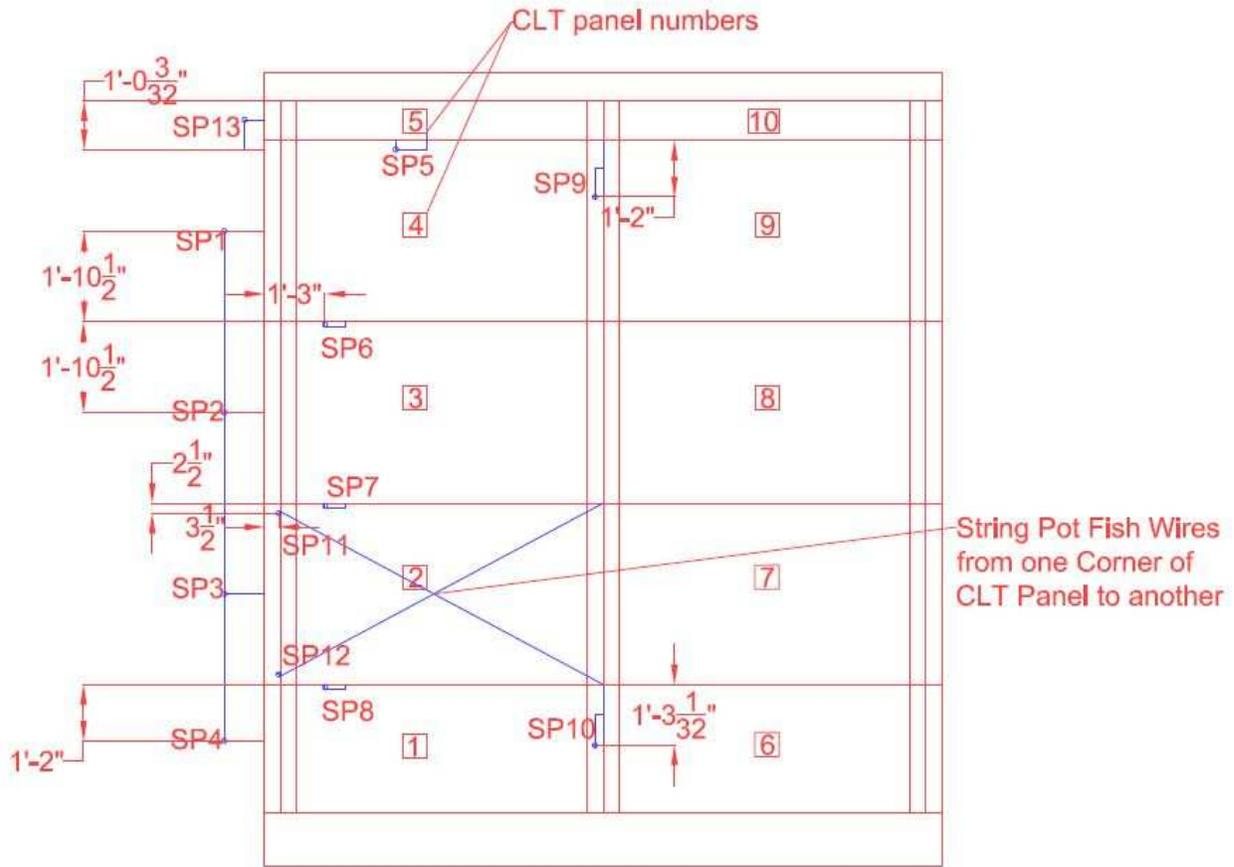
Figure 3.4 String Pot Locations on the CLT Diaphragm (Plan View)
