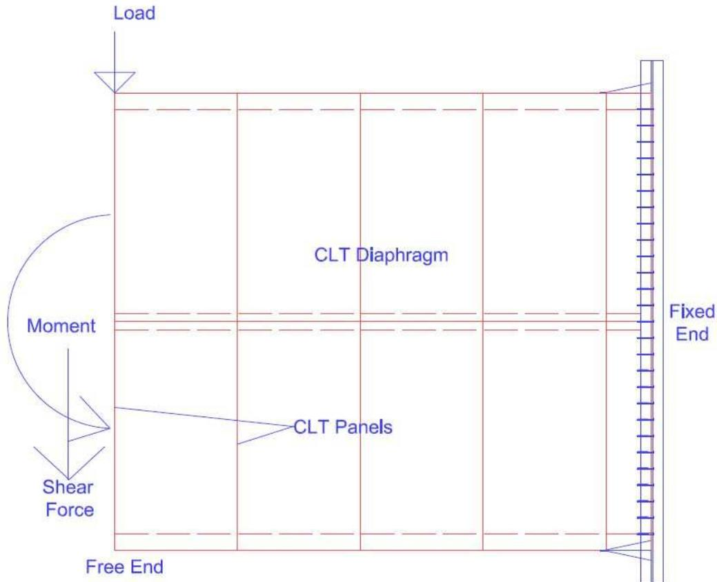
Figure 2.1 Cantilever Beam
