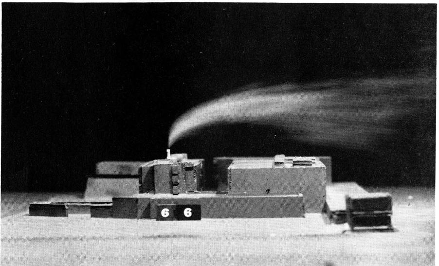
Figure 2. Plume visualizations for west (270°) wind.
