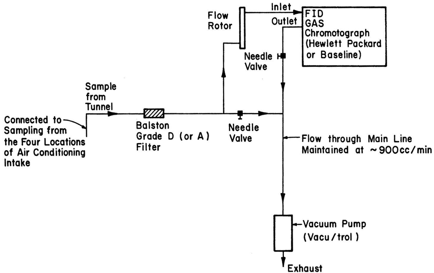
Figure 1.B. Schematic of gas sampling equipment set-up.
