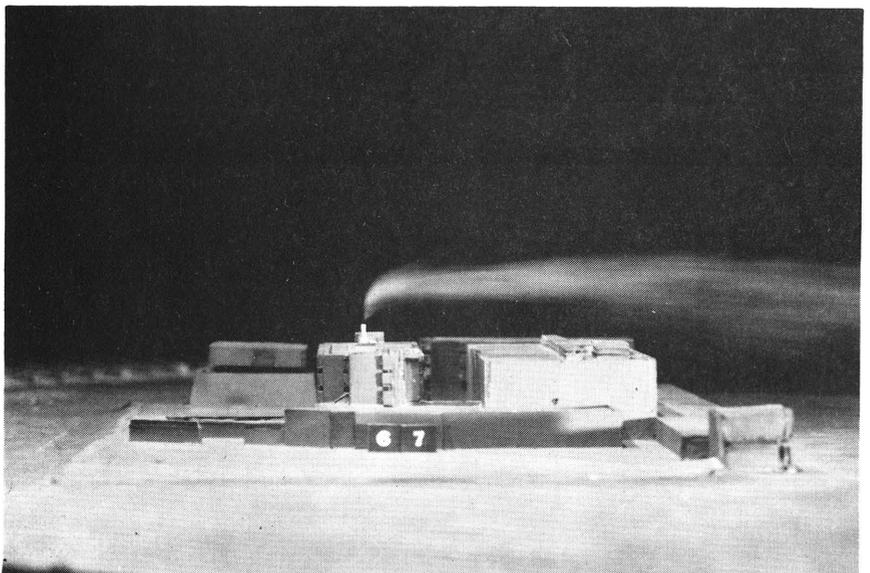
Figure 3. Plume visualization for northwest (315°) wind.
