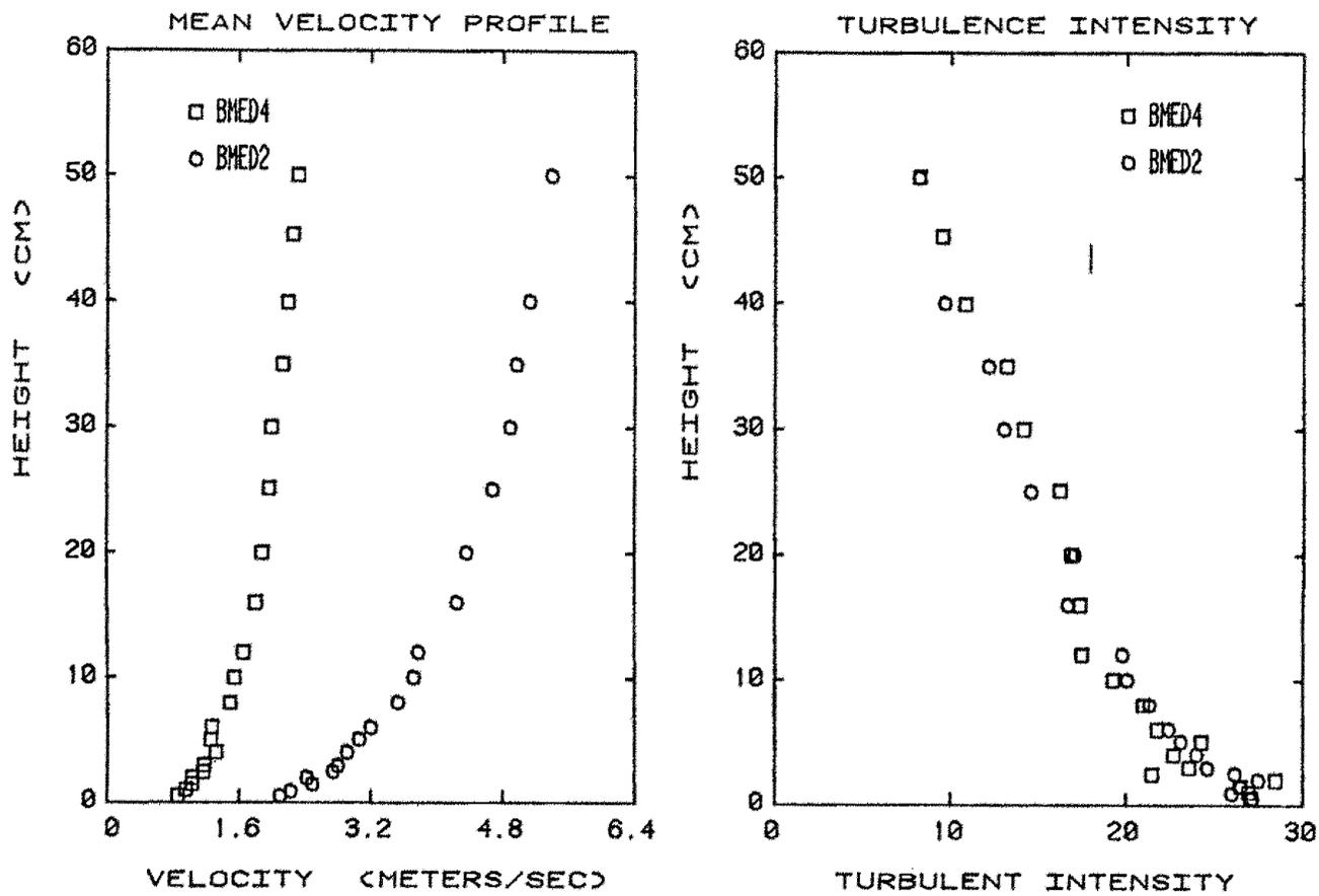
Figure 3.A. Mean velocity and turbulence intensity profiles.
