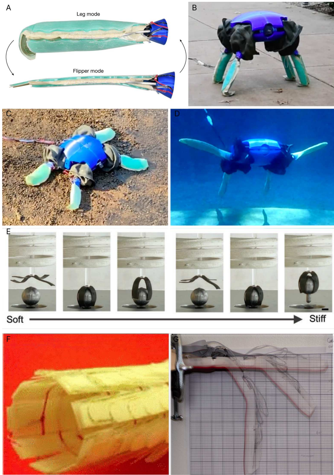
Figure 1.1: A) Side profile of morphing turtle leg [1]. B) Morphing turtle is capable of walking, C) crawling, and D) swimming [1]. E) Magnetic shape memory polymer is capable of varying stiffness to grasp objects [2]. F) Layer-jamming can be used to vary stiffness in surgical devices [3]. G) Thermoplastic composites with embedded actuators and sensor can localize stiffness variation [4].
