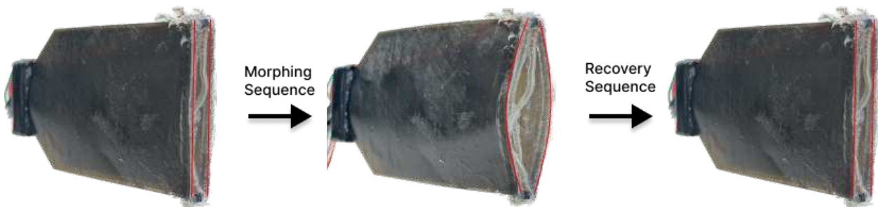
Figure 3.3: Morphing sequence of the shape-morphing tail. In the initial flat configuration, the tail has low stiffness. As TCA actuation curves the plates, stiffness increases, with the curved shape held in place by the SMP ribs. During the recovery sequence, as the SMP returns to its original state, the stiffness decreases.
