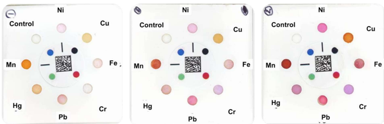
Figure 4. Representative images for spike recovery analysis showing on-card responses for lower to higher spiking concentrations (left to right).
