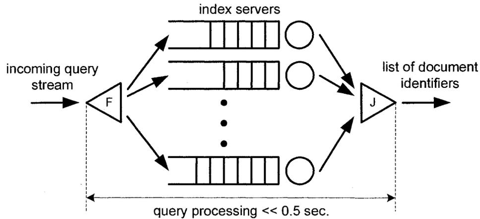
Figure 4.2: The Google example: Fork (F) and Join (J) query processing executed by index servers in the first phase of the search engine.
