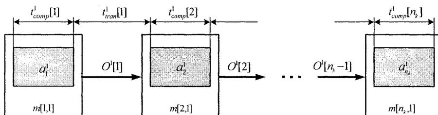
Figure 2.2: The string model for string 1. Shaded rectangles denote applications in the string while white rectangles represent the machines where these applications execute. The arrows represent output data transfers within the string.
