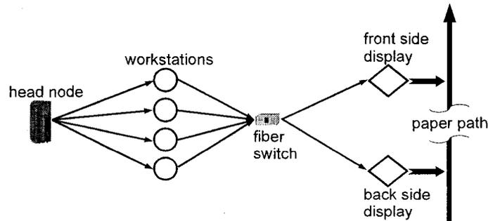
Figure 3.1: A conceptual model of a high performance, cluster-based imaging system.
