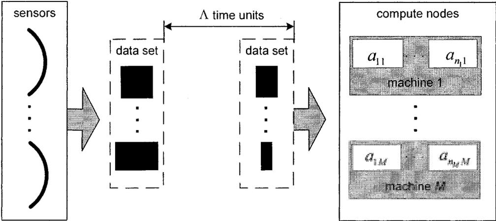
Figure 4.1: The CARA example: major functional units and data flow for a class of systems that operate on periodically updated data sets. The  $a_{ij}$ 's denote applications executing on machine  $j$ . Processing of each data set must be completed within  $\Delta$  time units.
