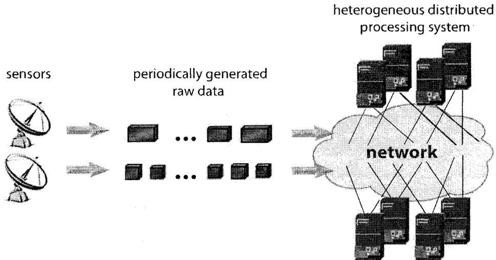
Figure 2.1: The considered part of the ARMS shipboard environment. Each sensor generates raw data periodically and forwards it to the distributed heterogeneous processing system.
