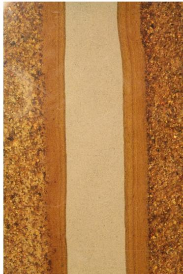
FIGURE 2.12. Post-treatment  $MnO_2$  deposits in the transmissive and low k soils in the permanganate treatment tank.
