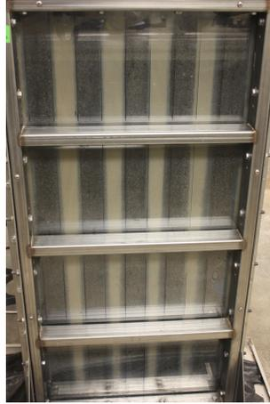
FIGURE 2.15. SRB, lactate and sulfate treatment at day 10 of the 27-day treatment (influent treatment solution was clear). Image shows deposition of black mineral phase in the transmissive and low k soils.
