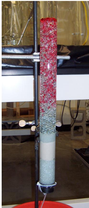
FIGURE 2.5. 1-m long TCE exchanger with dyed TCE in 6 mm glass beads, used to saturate influent water with TCE for delivery to tanks. Flow direction from bottom to top.
