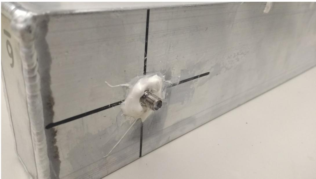
**Fig. 3.1.** Figures and photograph of the slotted-waveguide and the placement of the SMA connector as a probe.
