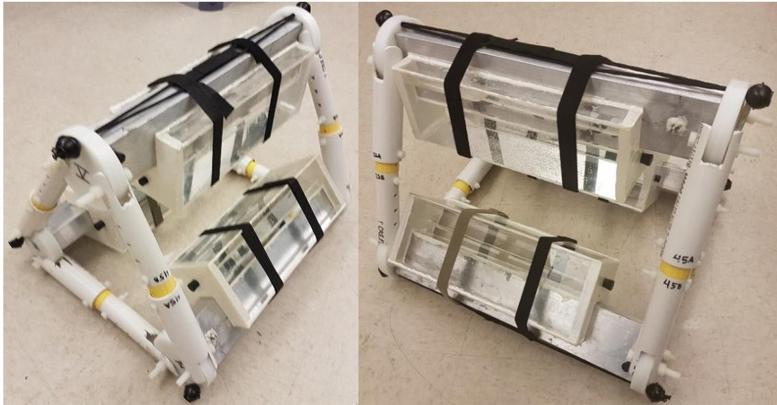
**Fig. 4.10.** The 3 element slotted waveguide array with dielectric lenses in extendable brackets.
