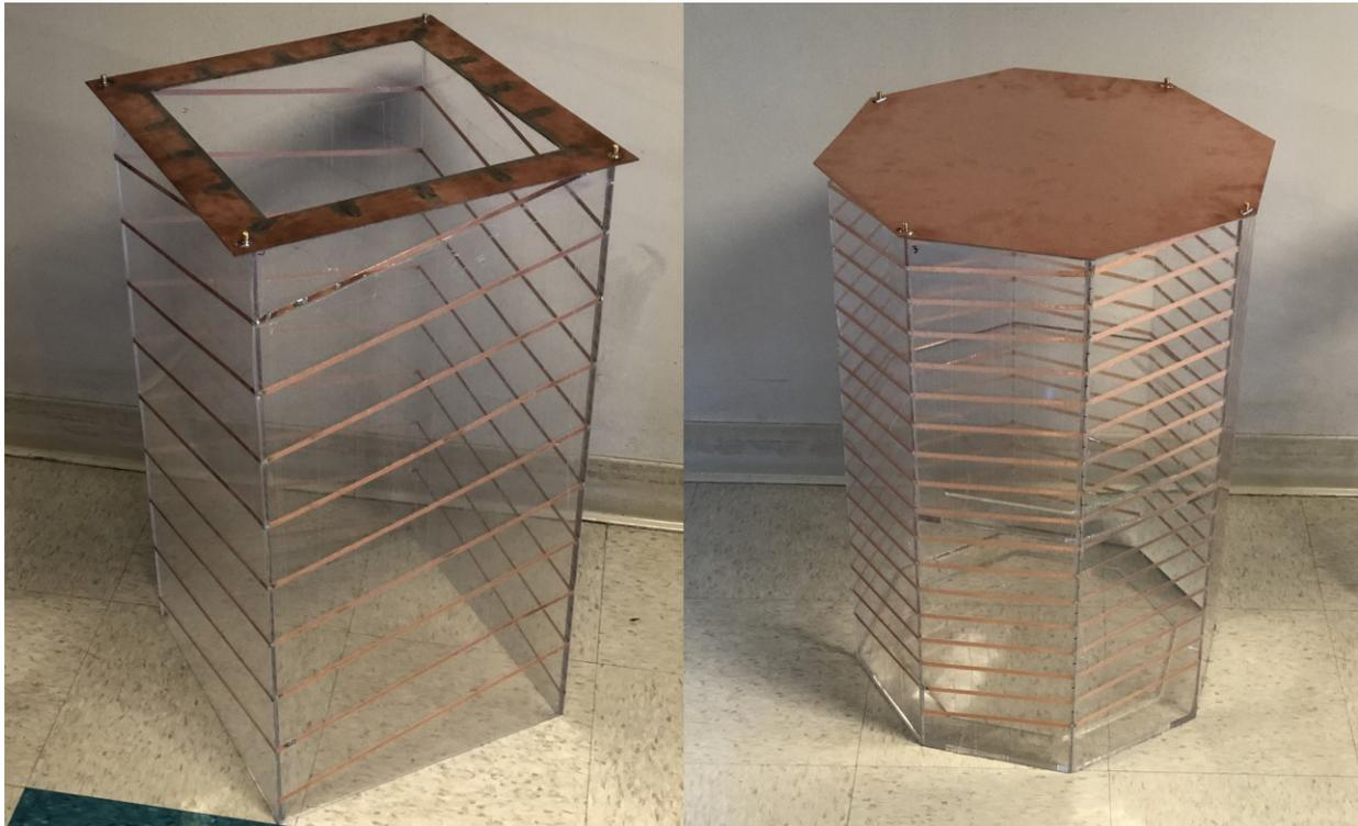
**Fig. 6.3.** Square-prism (left) and Octagonal-prism (right) quadrifilar helical RF coil prototypes.
