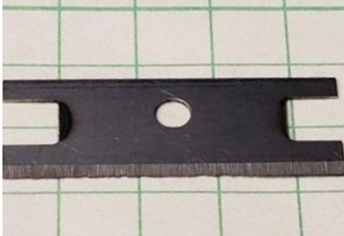
Figure 25: Damaged chopper gun blade.
