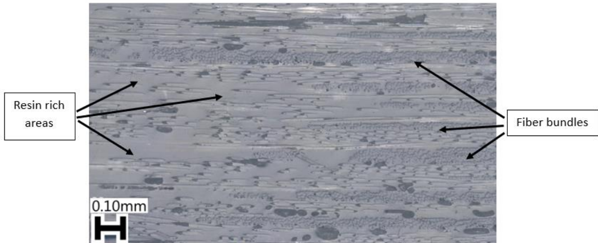
Figure 71: Fiber volume fraction gradient in specimen without any effects applied.
