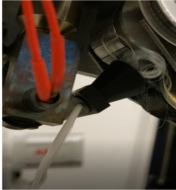
Figure 30: Tow guide bunching during refeed.
