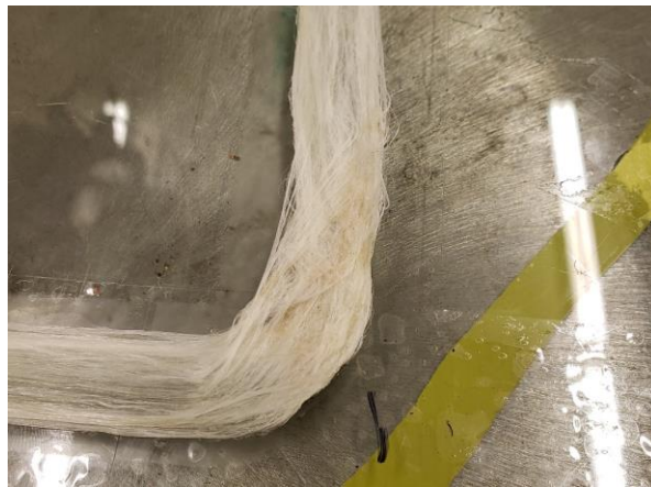
Figure 86: Fibers not tacking in corners.
