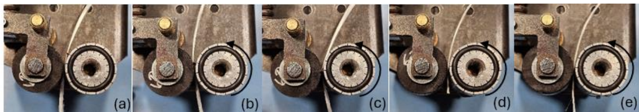
Figure 21: Cam is engaged, and fiber can be pulled through (a), tow is pinched (b), blade contacts tow (c), tow is severed and fed forward (d), finally, tow is refeed (e).
