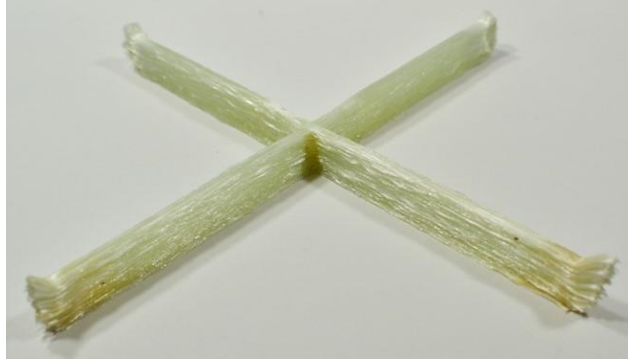
Figure 11: 40-layer stiffener grid intersection demonstration [53].
