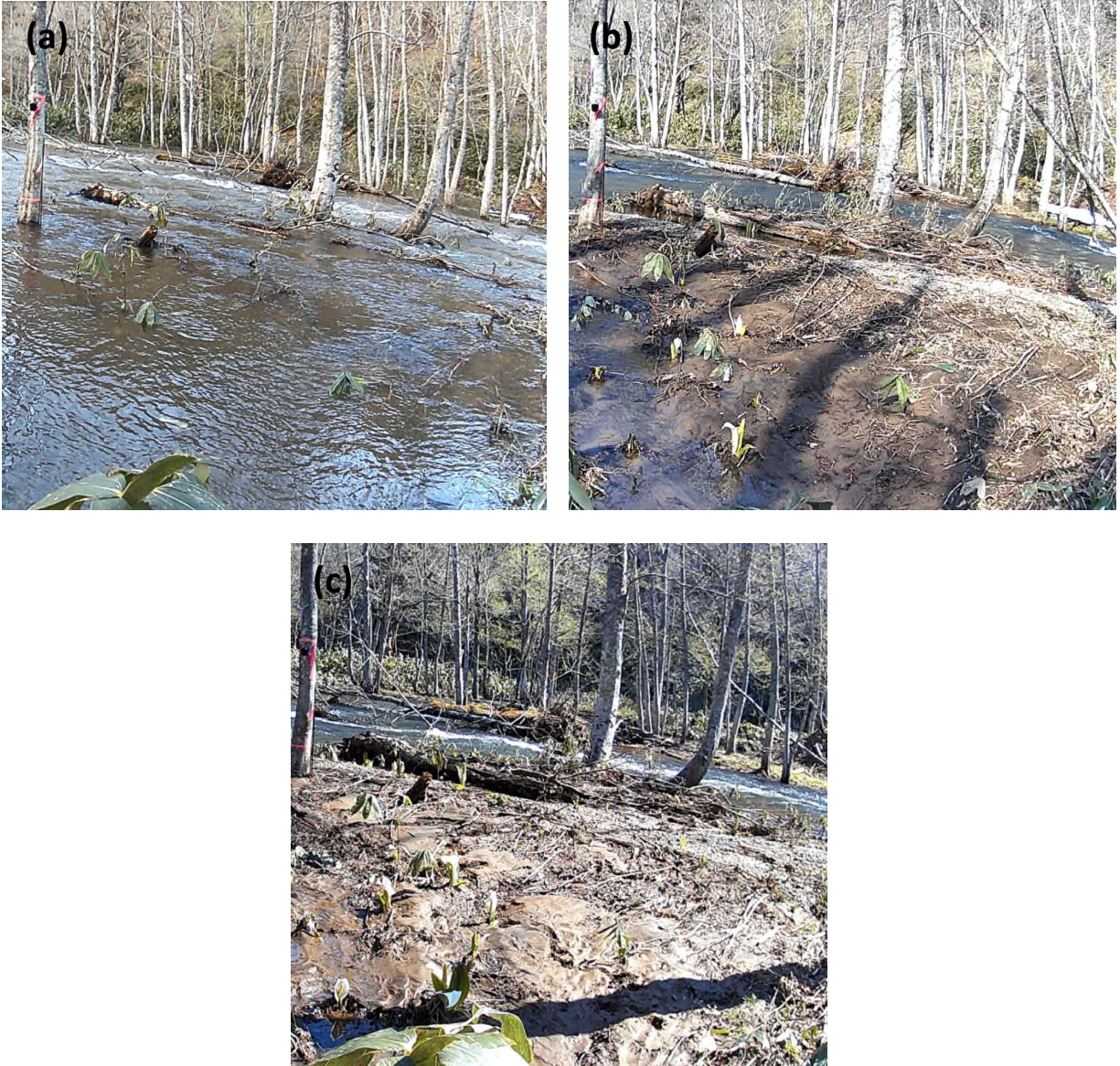
Figure 4.5. Photos from Reach 1 pointed toward a large side channel. This photo sequence shows an example of the methods described to calibrate the Manning’s coefficient values in the channel. In (a), taken 04 May 2022, the side channel is fully hydraulically connected. In (b), taken 05 May 2022, the channel is at the threshold of being fully hydraulically connected. This is the target stage identified to achieve a calibrated Manning’s roughness. In (c), taken 11 May 2022, there is no surface flow in the side channel.
