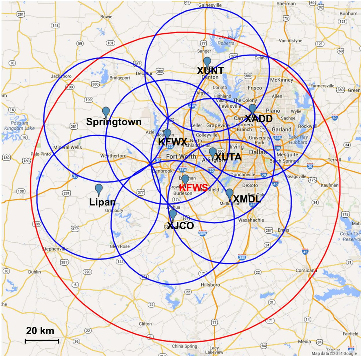
FIGURE 2.3. The CASA DFW Urban Testbed network of dual polarimetric X-band Doppler weather radars [1], plotted on Google Maps.
