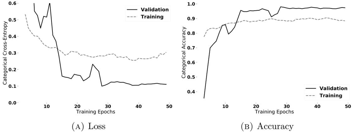
FIGURE 5.4. Loss and accuracy curves for our best-case network, which utilized the VGG16 base model feature extractor, with batch normalization layers following each convolutional layer, and BlurPool layers with a kernel size of 5. Training was allowed to progress with base model weights frozen until a loss plateau was reached, before fine-tuning by allowing all parameters to update during training. Fine Tuning began at Epoch 36.
