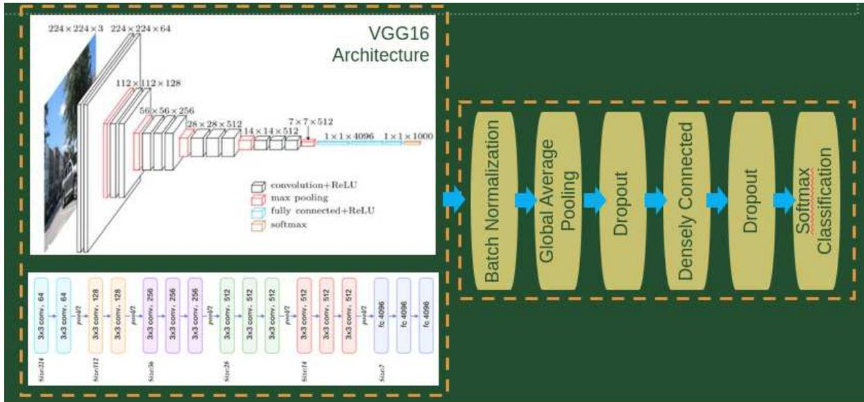
FIGURE 4.2. End-to-end deep learning architecture, with VGG16 convolutional base and bespoke top model.
