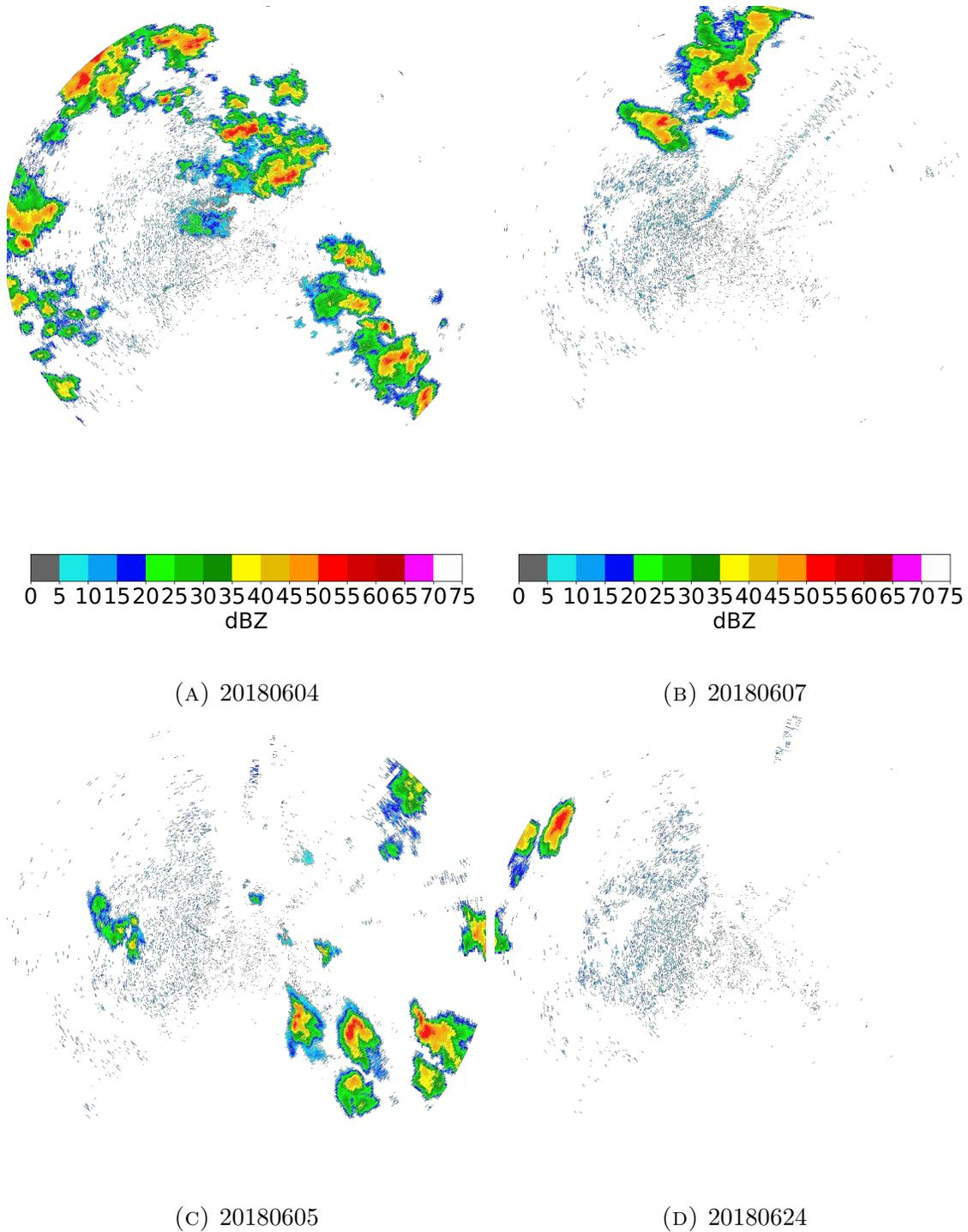
FIGURE 4.7. Example data that was discovered by model and labeled as convective precipitation. These scans were selected randomly from a large dataset from the month of June 2018, at the XMDL radar. Expert human curation is needed, though these four samples certainly represent the expected precipitation regime.
