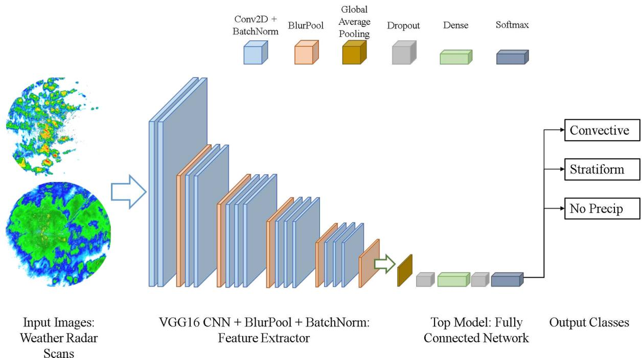
FIGURE 5.1. Complete end-to-end deep learning architecture devised in this chapter. Note that convolution layers now include batch normalization, while downsampling layers are formed by the new BlurPool layer. These two are tuneable parameters in this architecture, and we tested many configurations to find the best set of parameters and hyperparameters.
