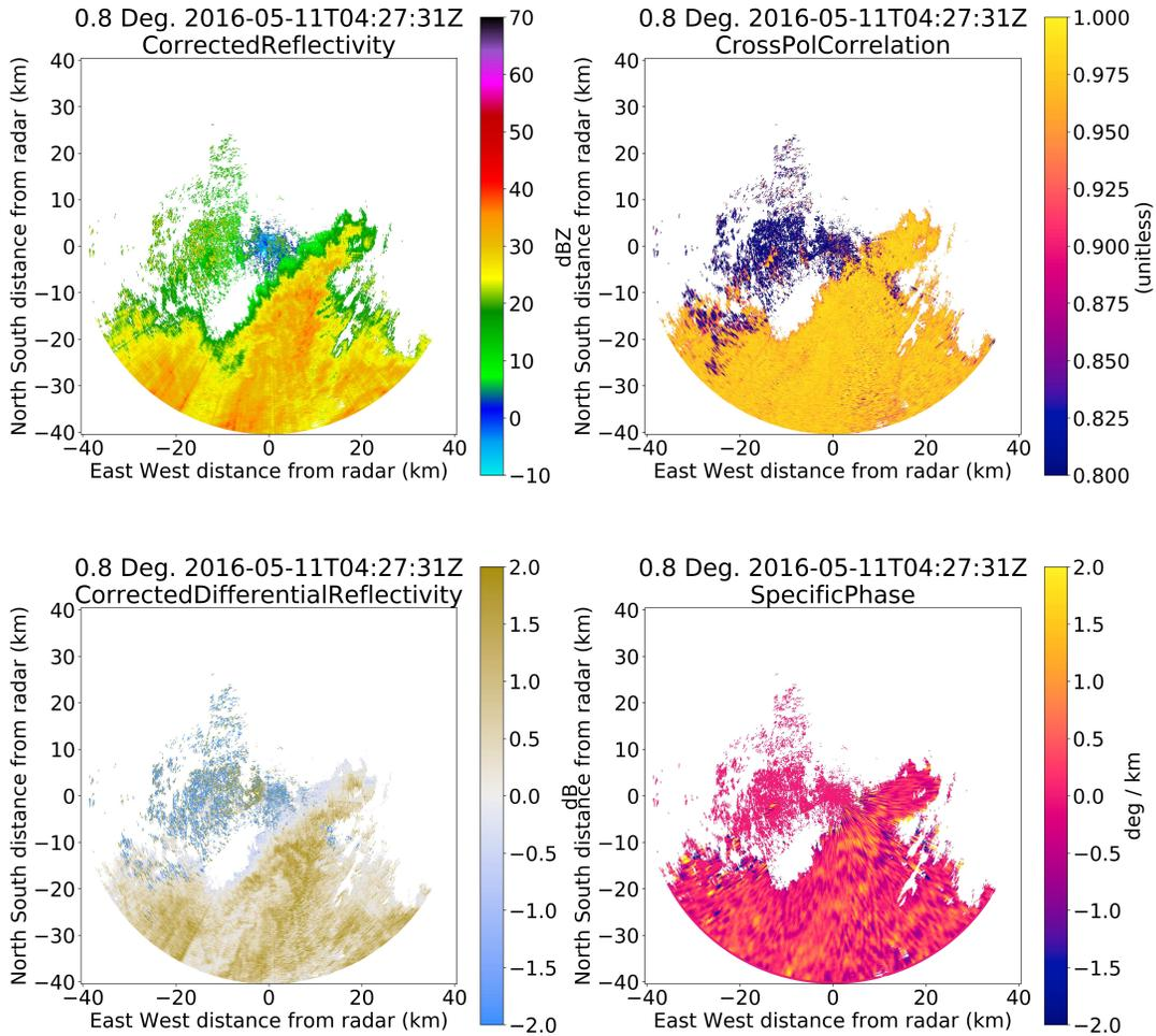
FIGURE 2.1. Examples of radar variables, left to right, top to bottom:  $Z_h$ ,  $\rho_{hv}$ ,  $Z_{dr}$ , and  $K_{dp}$ . Case from 2016-05-11, XMDL Radar, CASA DFW network. This particular scan is from the stratiform precipitation regime, as evidenced by relatively low  $Z_h$ , high  $\rho_{hv}$ , and middling  $Z_{dr}$ .
