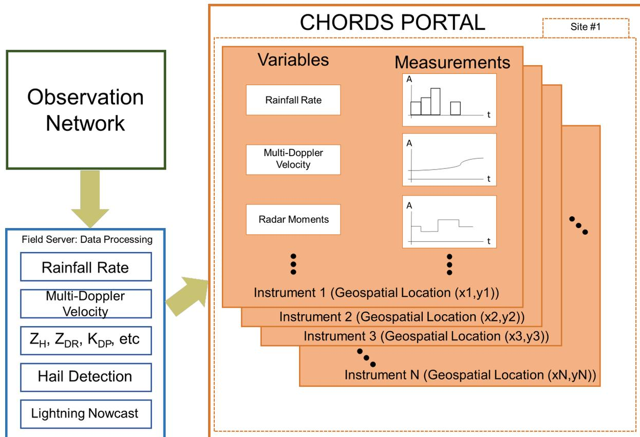
FIGURE 6.1. CHORDS Portal, where selected radar range gates are used as Variables, allowing collocated ground sensors to stream data and provide direct ground-to-radar validation in real-time
