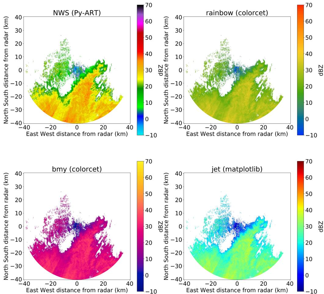
FIGURE 2.2. Examples of colormaps. Case from 2016-05-11, XMDL Radar, CASA DFW network. Variable plotted is Corrected Reflectivity  $Z_h$ . Notice how in the perceptually uniform colormaps 'rainbow' and 'bmy' that it is easier to quickly detect textures within the precipitation regions of the image. The NWS colormap draws the eye to the red regions, which correspond to higher reflectivities, and 'jet' fails to do either.
