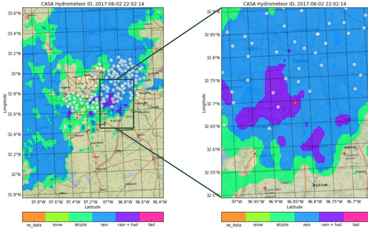
FIGURE 6.2. Aligning hydrometeor identification product with hail sensor hits in the Dallas Fort Worth area, illustrating an example CHORDS use case
