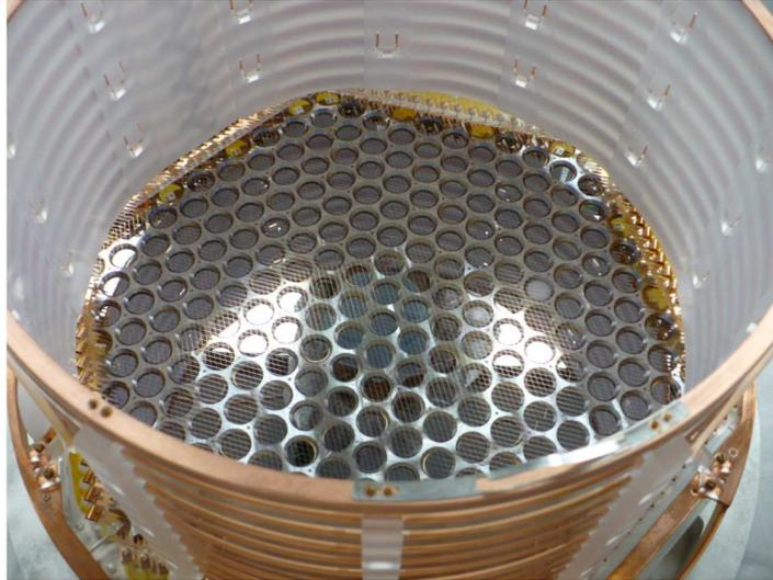
**Figure 1.9:** This picture shows the holes into which the LAAPDs were be mounted. The wire planes are already installed in front of the holes. The top of the cylinder is the cathode plane, though the cathode was not yet installed.
