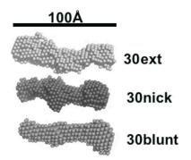
**Supplementary Figure 7.** *Ab initio* models of 30ext, 30nick and 30blunt DNA samples. The models were calculated from the average of ten DAMMIN *ab initio* models. The DNA models are all between 88-100Å in length, and cannot be differentiated from either B or A form DNA given the resolution of the technique.
