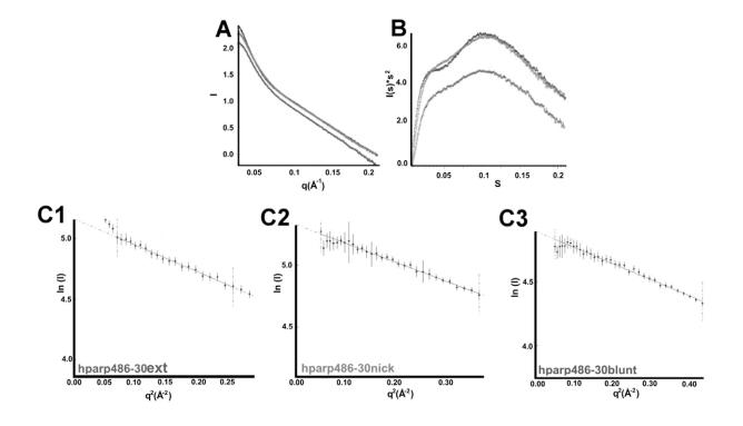
Supplementary Figure 4.8. Analysis of SAXS data for parp486 in complex with blunt, nicked and 6n3' DNA. A) Raw SAXS scattering for each protein-DNA complex. B) Kratky analysis of the complexes reveals an overall similar profile. C1-C3) Guinier analysis of each complex reveals that the data are devoid of aggregation.
