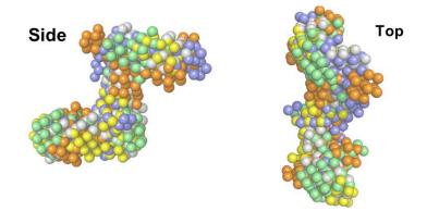
Supplementary Figure 2. Superposition of *ab initio* SAXS models of hparp486. The side (left) and top (right) views of five of the thirty averaged models that were used to create the final hparp486 particle reconstruction are shown. Each model is represented in a unique color. While the models do differ in certain areas, the overall shape of the particle remains similar. These models fit the SAXS scattering profile with a final  $\chi$ 2 between 1.05-1.15.
