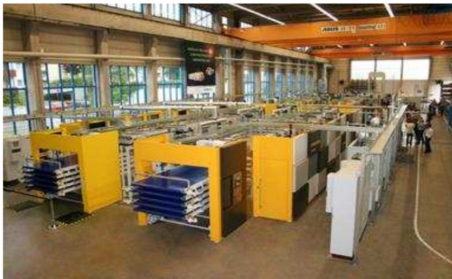
Fig. 5.5: Production type vacuum laminator. Note the scale of the people on the right side of the picture [Rimas].
