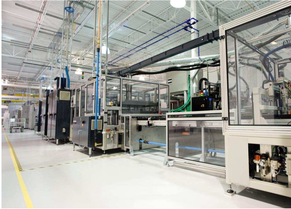
Figure AIII.3: Photograph of the high throughput encapsulation fabrication tools at Abound Solar's Longmont Colorado facility. These automated manufacturing systems could process one module in under 30 seconds.
