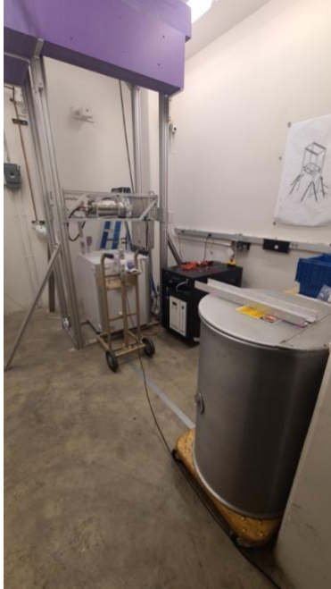
Figure 16. Bonner Sphere system at 1 m distance from unshielded PuBe source in MRB 002.
