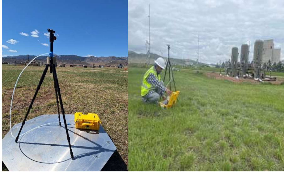
Figure 2.3. Example of a field deployment of methane concentration sampling. The tubing inlet connected to the gas analyzer (MGGA) and mounted to the tripod at 1 m above the ground level.
