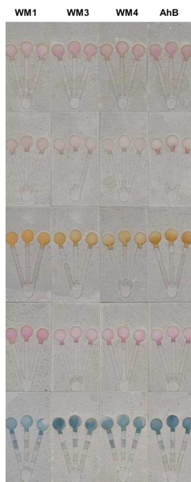
Figure S1. Photograph showing color changes for different paper substrates, including Whatman 1, Whatman 3, Whatman 4, and Ahlstrom blotting paper, used in the detection of (a) Ni, (b) Fe, (c) Cu, (d) NO 2 - , and (e) PO 4 3- .
