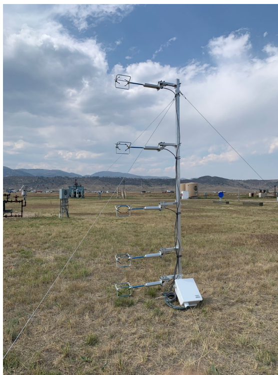
Figure A1. An anemometer array consisting of five, 3D sonic anemometers.
