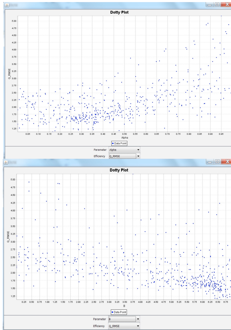
Figure 7. Dotty plots of RMSE vs. HyMod \alpha and \beta parameter values resulting from 1000 uniform random samples of the parameter space.
