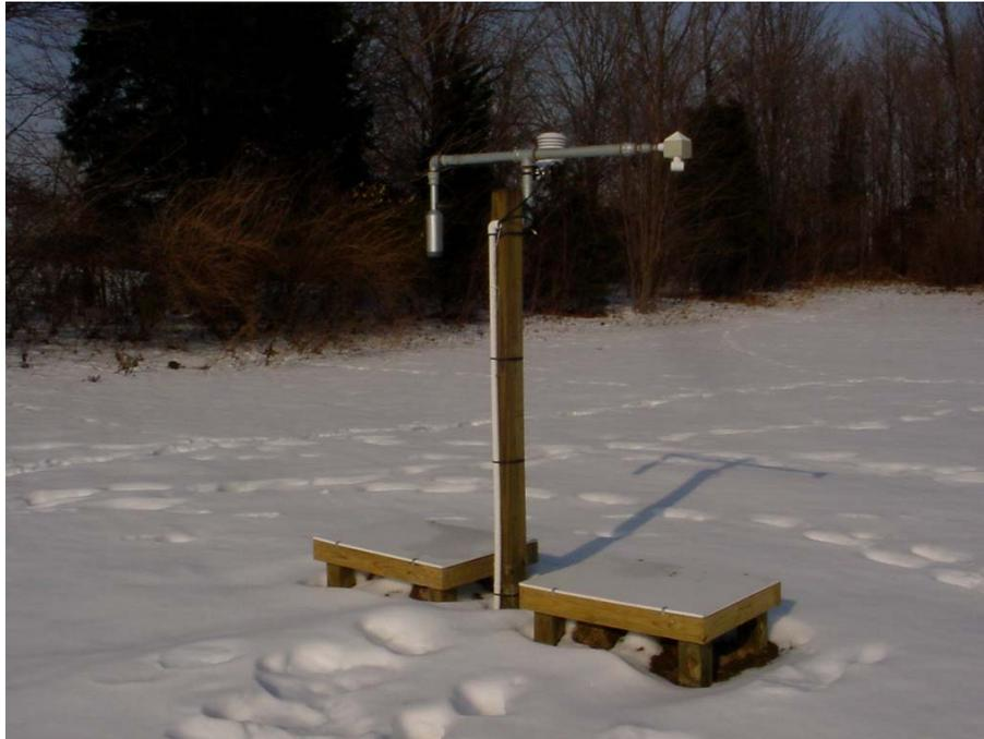
Figure 5-1: Site setup in Indianapolis, IN caused excessive wind scour and melting of the snow beneath the sensors.
