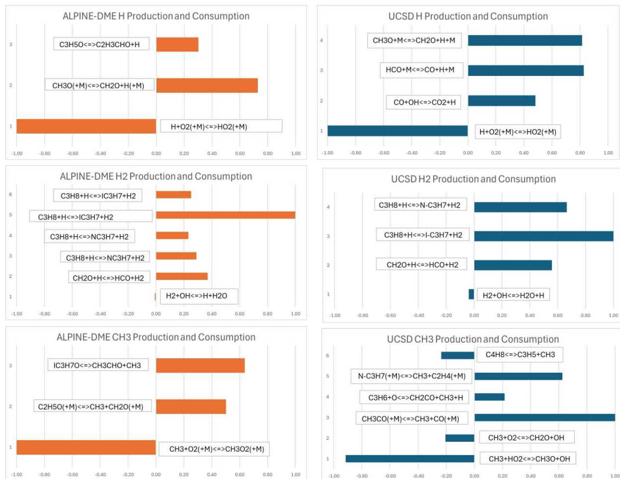
Figure 6.13 Ignition delay species sensitivity analysis normalized ROP for H, H 2 , and CH 3 at 0.5% induction offset for 100% Propane at 690K and 30 bar between two chemical kinetic mechanisms UCSD and ALPINE-DME 158.
