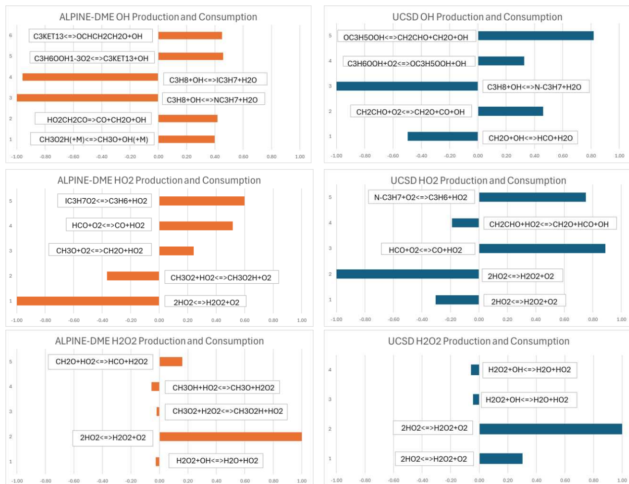
Figure 6.12 Ignition delay species sensitivity analysis normalized ROP for OH, HO 2 , and H 2 O 2 at 0.5% induction offset for 100% Propane at 690K and 30 bar between two chemical kinetic mechanisms UCSD and ALPINE-DME 158.
