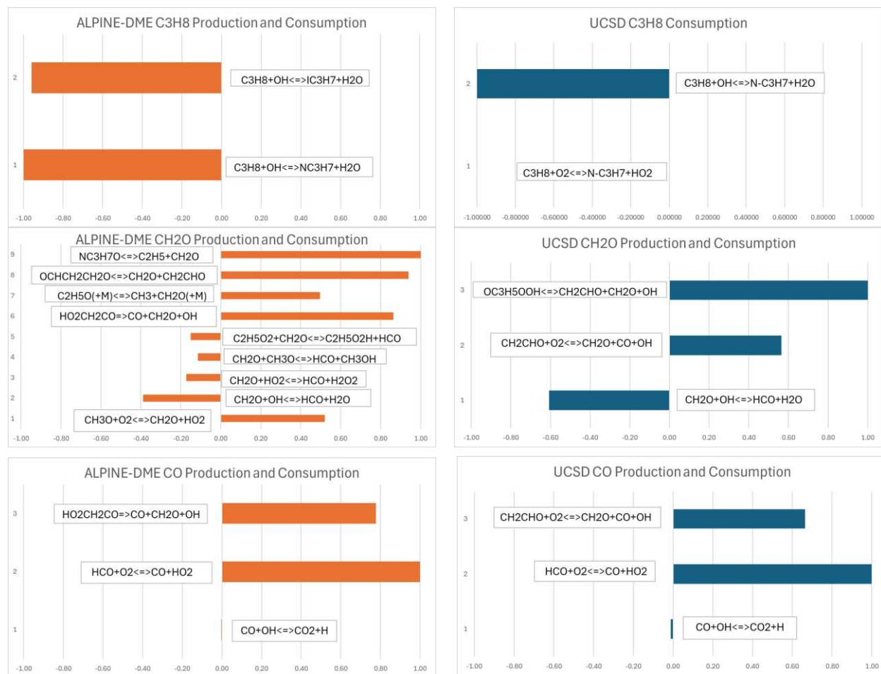
Figure 6.14 Ignition delay species sensitivity analysis normalized ROP for C 3 H 8 , CH 2 O, and CO at 0.5% induction offset for 100% Propane at 690K and 30 bar between two chemical kinetic mechanisms UCSD and ALPINE-DME 158.
