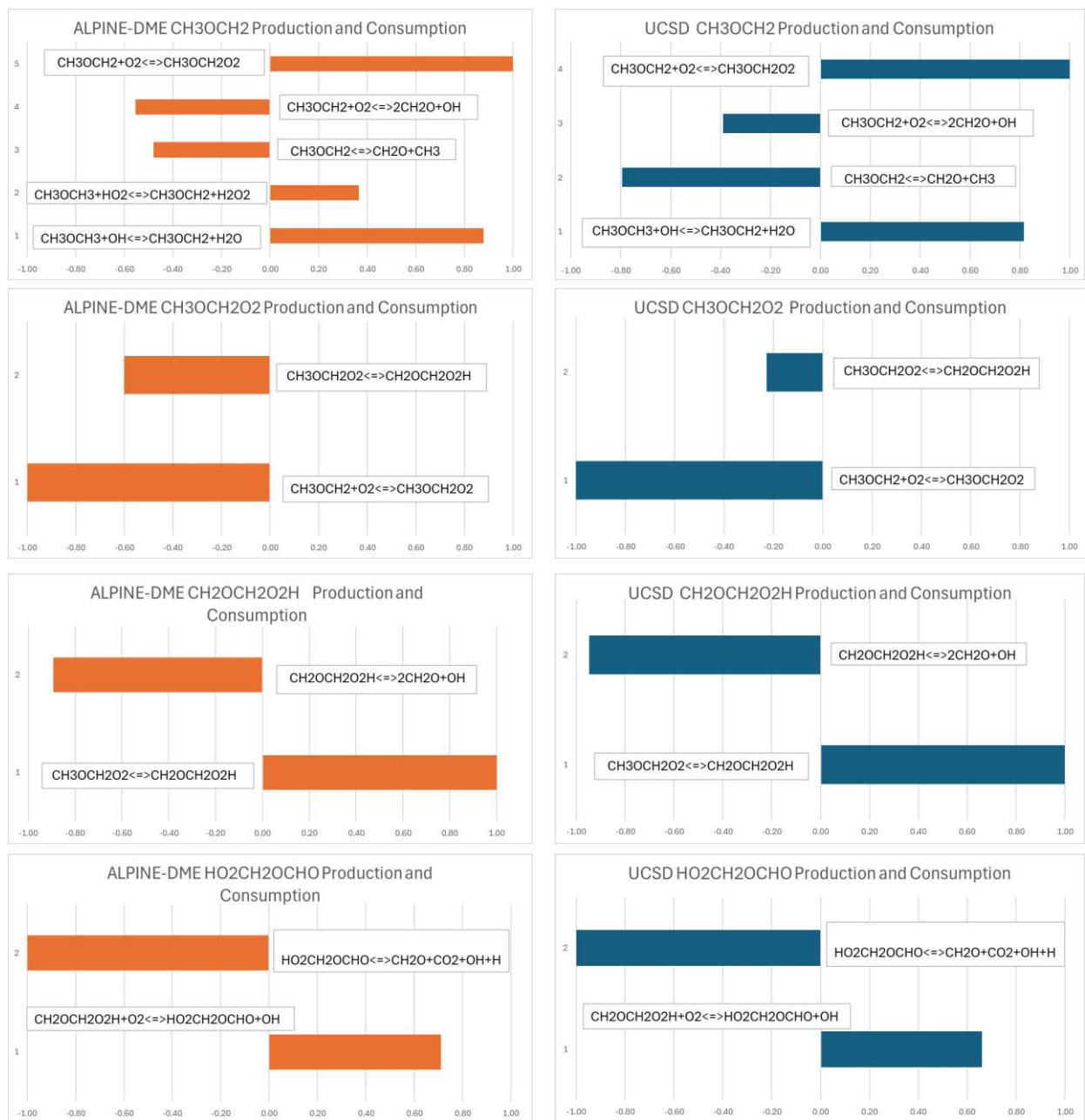
Figure 6.18 Ignition delay species sensitivity analysis normalized ROP for \text{CH}_3\text{OCH}_2 , \text{CH}_3\text{OCH}_2\text{O}_2 , \text{CH}_2\text{OCH}_2\text{O}_2\text{H} , and \text{HO}_2\text{CH}_2\text{OCHO} at 0.5% induction offset for 75% Propane and 25% DME at 690K and 30 bar between two chemical kinetic mechanisms UCSD and ALPINE-DME 158.
