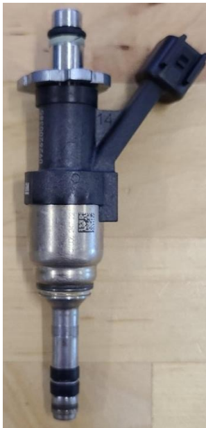
Figure 3.14. Image of the XDI injector and the results from the mass flow rate vs injection pressure sweep comparison of DI injectors.
