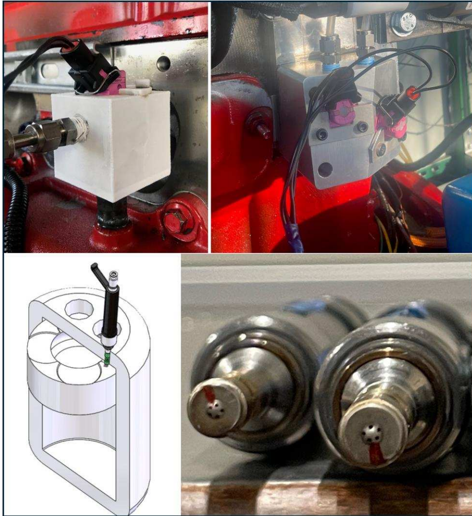
Figure 2.2. L-R A picture of the Siemens DEKA port-fuel injector installed in the baseline configuration of the engine, the double-injector valve-targeting PFI set-up for the higher compression ratio engine configuration, a CAD model of the direct injector imposed in the cylinder, and the modified direct injectors.
