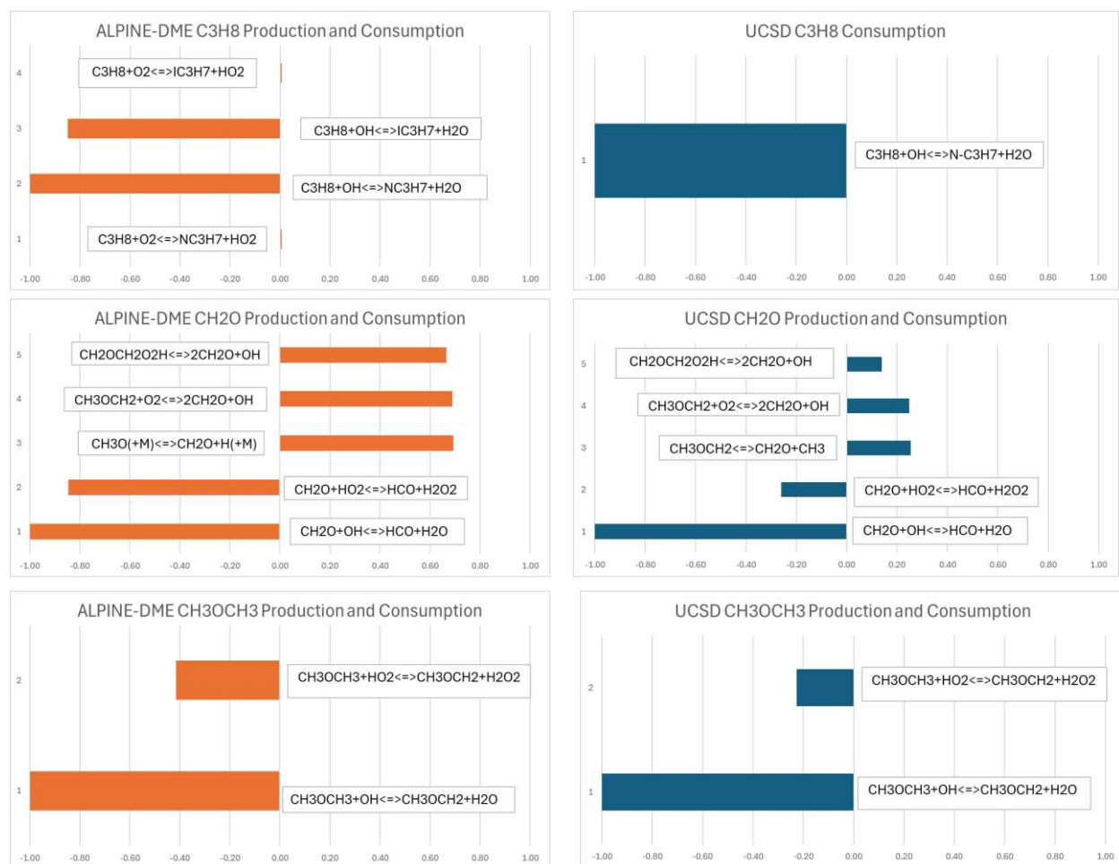
Figure 6.17 Ignition delay species sensitivity analysis normalized ROP for C 3 H 8 , CH 2 O, and CH 3 OCH 3 at 0.5% induction offset for 75% Propane and 25% DME at 690K and 30 bar between two chemical kinetic mechanisms UCSD and ALPINE-DME 158.
