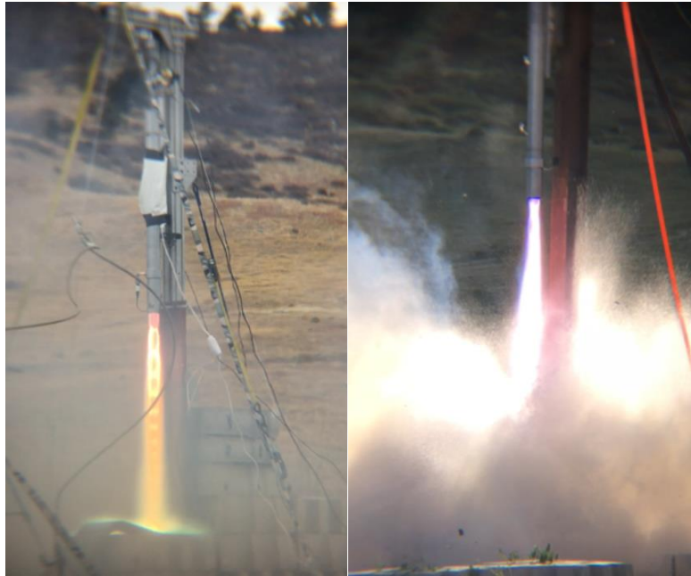
Figure 2-9. Hot test fires of previous motors using nitrous oxide at Colorado State University.
