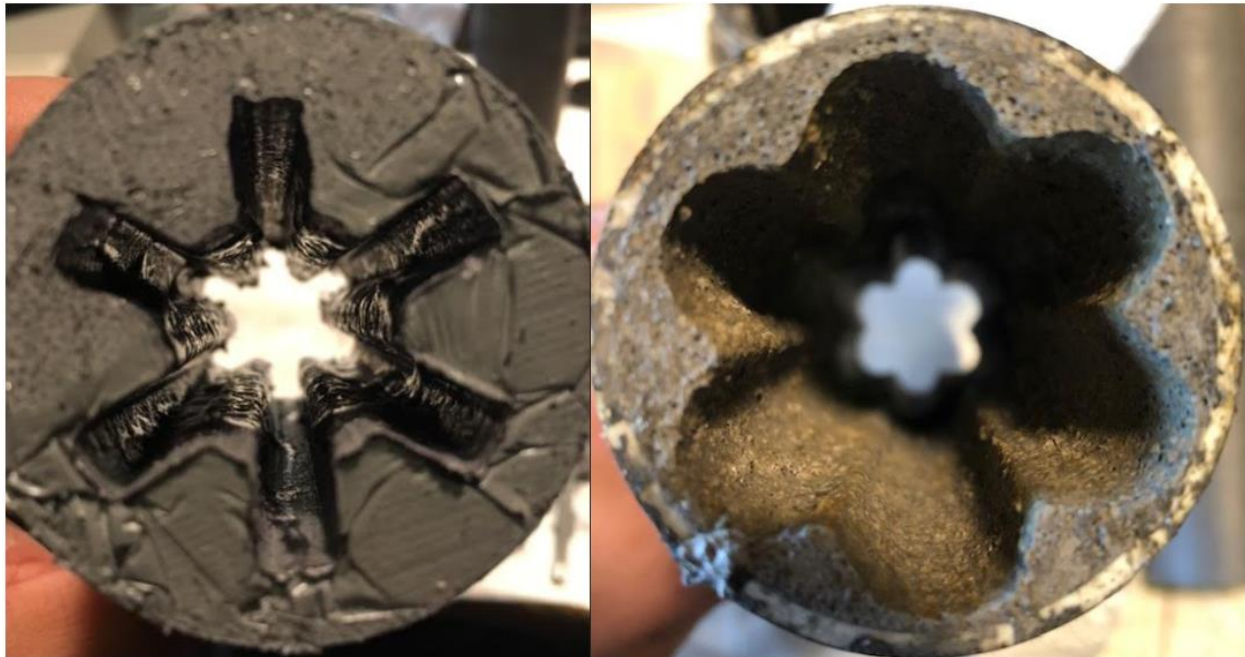
Figure 4-34. Test Fire 5 fuel grain before (left) and after (right) hot test firing.
