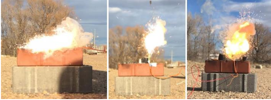
(a) (b) (c) Figure 3-2. Ignition testing of Ignitor-1 (a), Ignitor-2 (b), Ignitor-3 (c).
