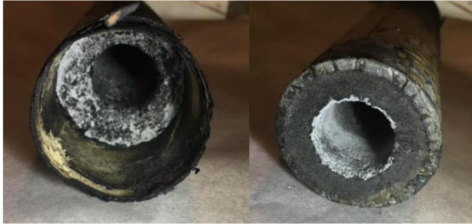
Figure 4-16. Injector side (left) and nozzle side (right) of the grain post-firing.
