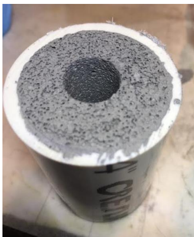
Figure 4-8. Paraffin wax in test fuel grain.
