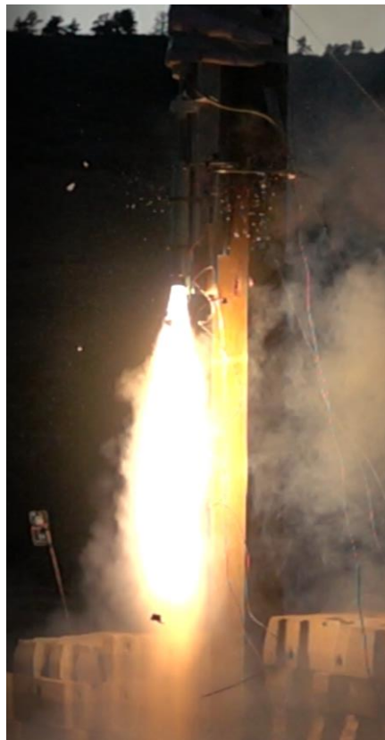
Figure 4-27. October 3 rd hot fire test: 50% nitrous oxide and 50% carbon dioxide.
