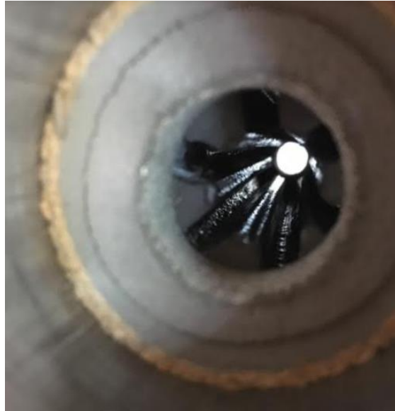
Figure 4-18. View of preheater grain looking towards the finocyl fuel grain.
