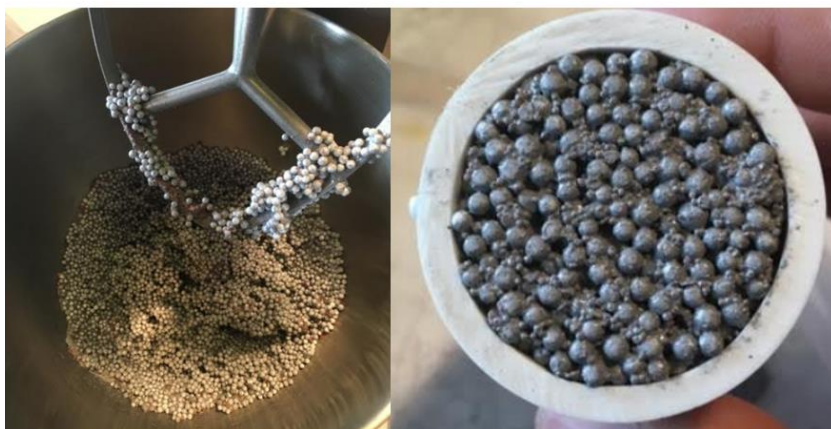
Figure 4-7. Styrofoam beads in test fuel grain.
