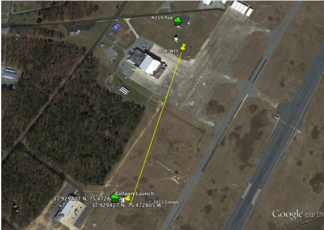
FIGURE 5.3. Radar calibration setup at Wallops Flight Facility. D3R system indicated by yellow pin on top and calibration tower located at bottom yellow pin.
